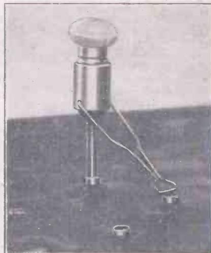
*This useful device, made by the Jeb Trading Co., can be used for testing batteries and valve-socket connections.*
