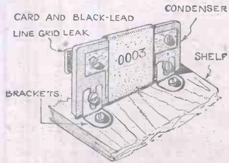
Fig. 4.—Condenser Mounting.
