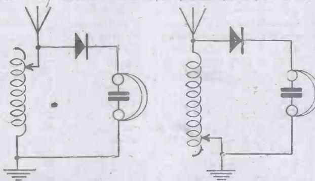
Figs. 3a and 3b.—Two Simple Crystal Circuits.
