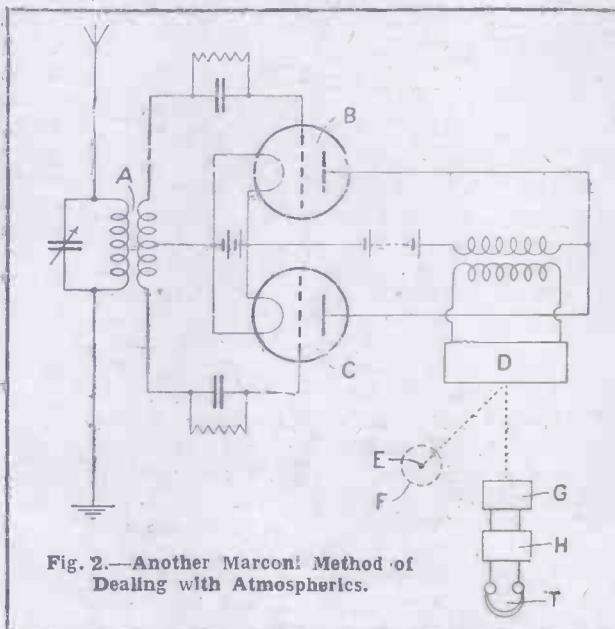
Fig. 2.—Another Marconi Method of Dealing with Atmospherics.
