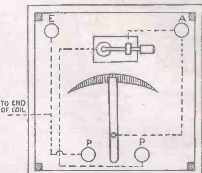
Fig. 2.—Plan of Panel with Wiring.
