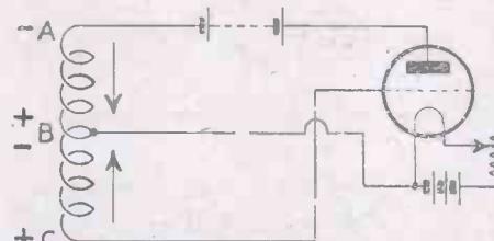
Fig. 20.—Principle of Valve Transmitter.
