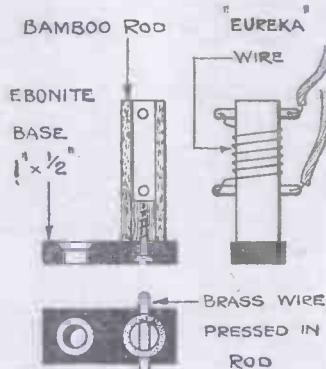
Fig. 6.—Details of Fixed Resistance.
