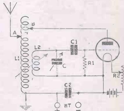
Fig. 21.—Circuit Diagram of Single-valve Transmitter.
