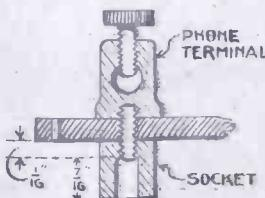
Fig. 4.—Details of Terminal and Socket.
