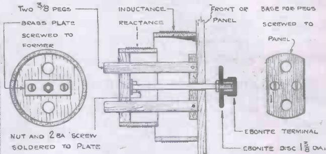
Fig. 5.—Arrangement of Tuning Coils.
