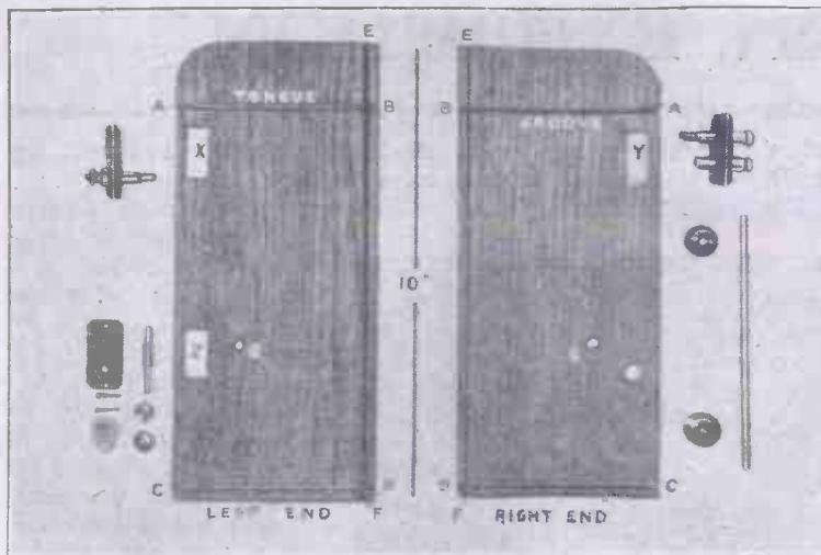
Fig. 1.—Cabinet Ends with Aerial, Earth and Telephone Terminals.
