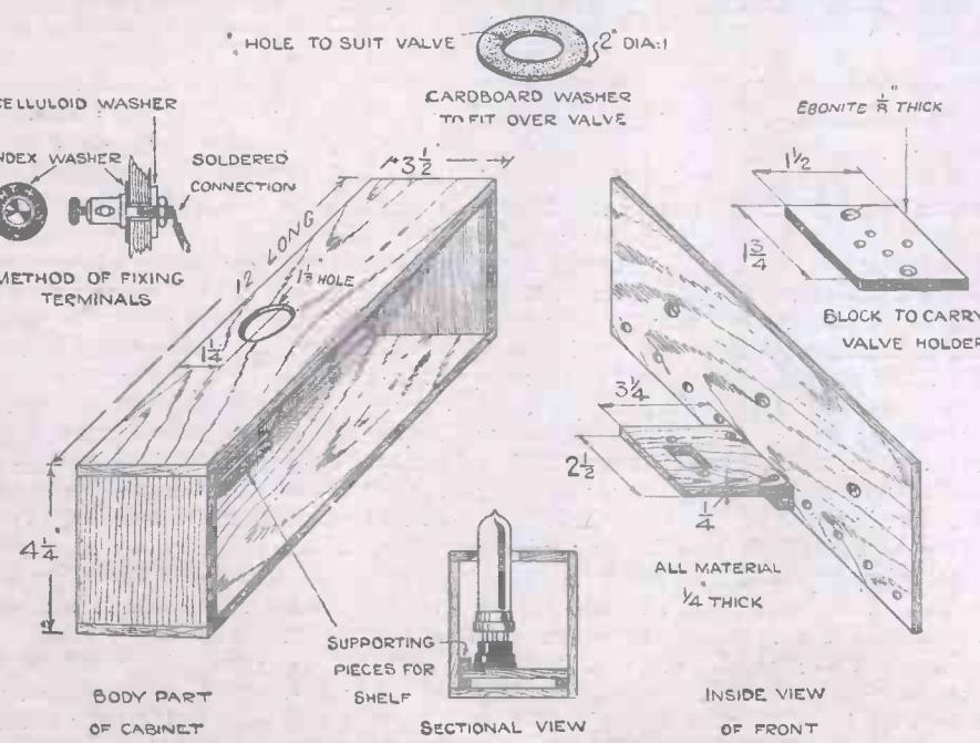
Fig. 1.—Details of the Cabinet and Valve Mounting.
