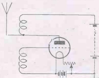
Fig. 19.—A Simple Valve Oscillator.
