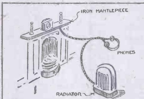
Fig. 2.—A Receiver for 2LO at a distance of a quarter of a mile.
