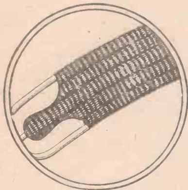
The headbands are made of piano wire covered in soft, corded webbing. At both ends the wire is firmly clamped together so that the original shape may be easily bent to fit the natural line of the head without fear of injuring the headband. They mean comfort without hard and irritable constriction.
