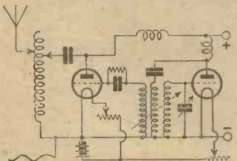
Fig. 40.—A Typical Master-oscillator.
