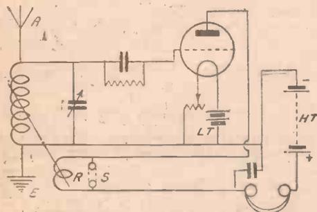
Fig. 1.—Typical Single-valve Circuit.
