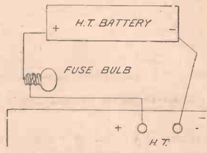
Fig. 3.—Method of Connecting Fuse.
