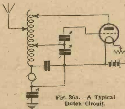
Fig. 36a.—A Typical Dutch Circuit.
