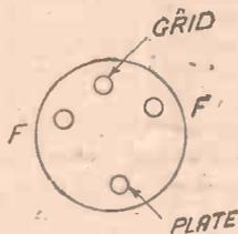
Fig. 2.—Valve Connections.
