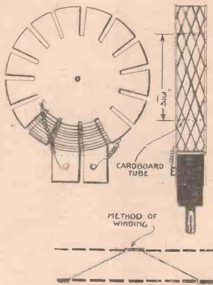
Method of Winding Coils.
