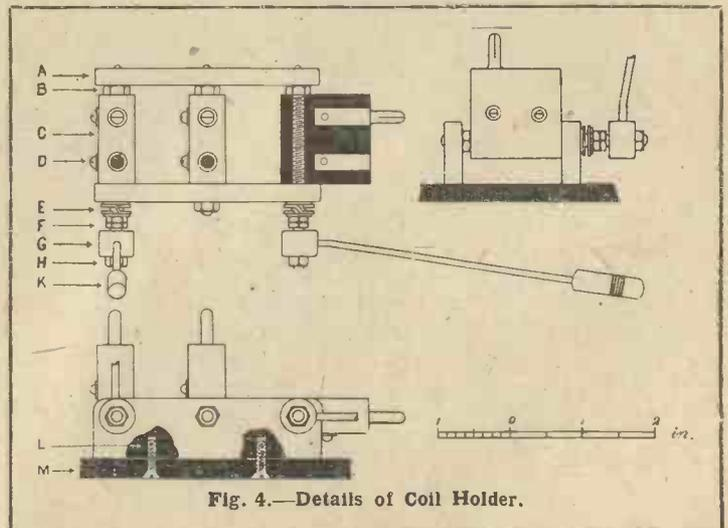
Fig. 4.—Details of Coil Holder.
