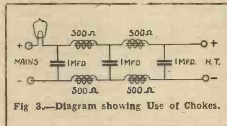
Fig. 3.—Diagram showing Use of Chokes.
