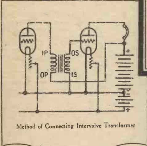
Method of Connecting Intervalve Transformer
