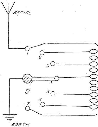
Fig. 1.—Diagram of Variable Inductance Connected to Aerial.
