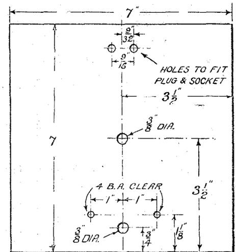
Fig. 2.—Lay-out of Panel.
