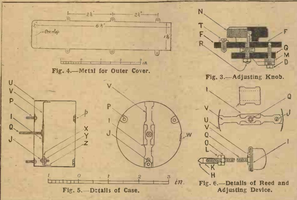
The outer cover can be made out of a strip of brass sheet cut according to the dimensions given in Fig. 4, which is rolled round and the joint W (Fig. 5) soldered. For fixing this to the receiver and the magnets, nuts are soldered on the inside of the three projections of one side, while small 6 B.A. screws P are soldered on the opposite three projections (see Fig. 5).
