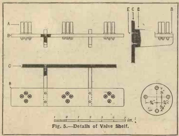
Fig. 5.—Details of Valve Shelf.
