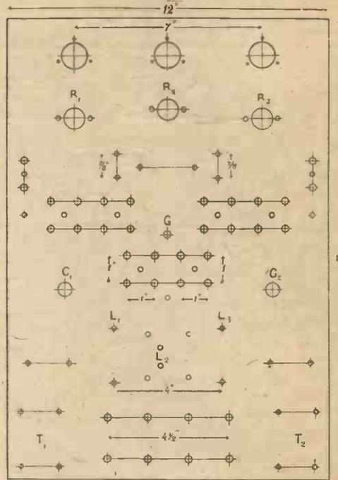
Fig. 3 (above).—Drilling Layout of Panel.
