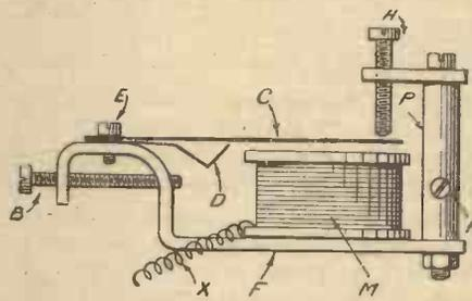
Fig. 5.—Details of Buzzer.
