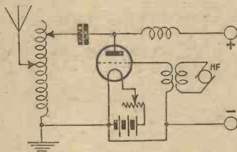
Fig. 37 — The Principle of the Master-oscillator.
