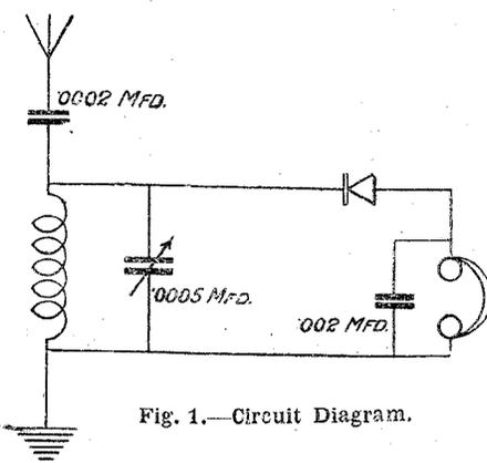
Fig. 1.—Circuit Diagram.
