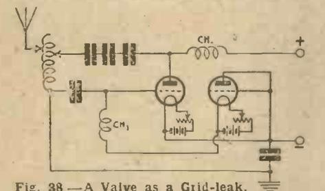
Fig. 38 — A Valve as a Grid-leak.
