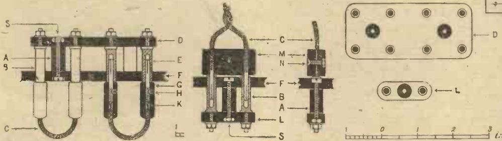
Fig. 6 (left).—Details of Plugs and Socket.
