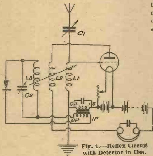
Fig. 1.—Reflex Circuit with Detector in Use.
