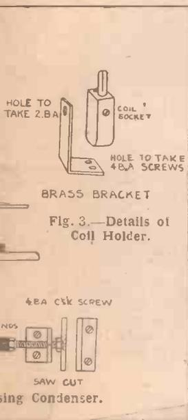
Fig. 3.—Details of Coil Holder.
