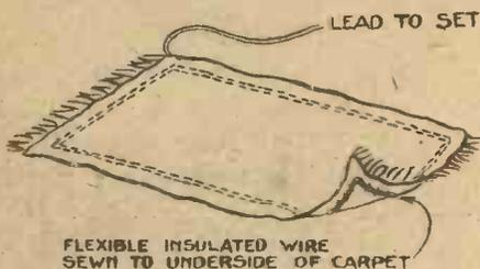
FLEXIBLE INSULATED WIRE SEWN TO UNDERSIDE OF CARPET
