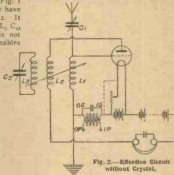
Fig. 2.—Effective Circuit without Crystal.
