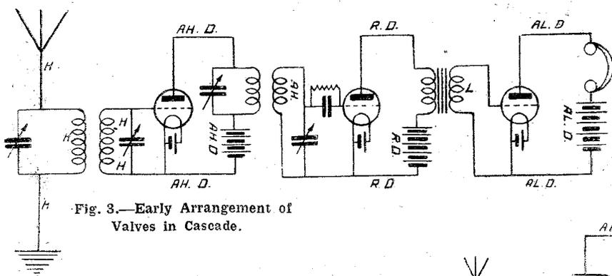
Fig. 3.—Early Arrangement of Valves in Cascade.
