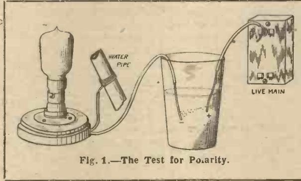
Fig. 1.—The Test for Polarity.
