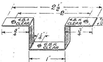
Fig. 3.—Buzzer Bracket.
