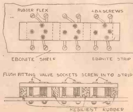
Fig. 6.—Details of Valve Holder.
