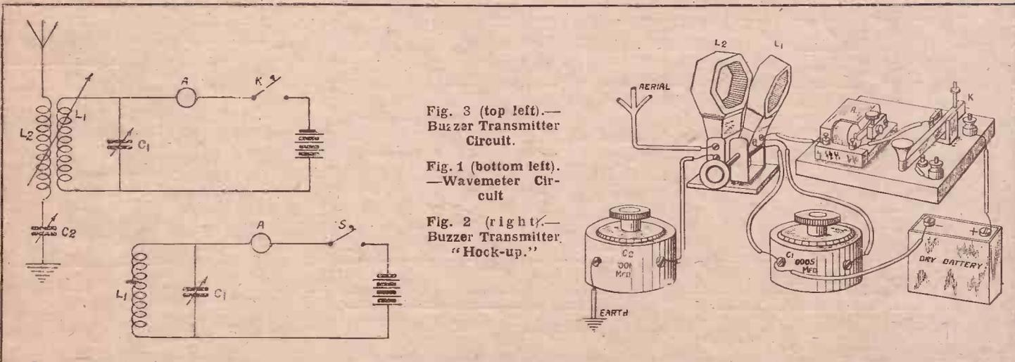
Fig. 3 (top left).—Buzzer Transmitter Circuit.
