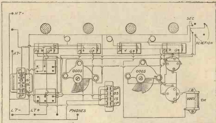
Fig. 3.—Wiring on Under Side of Panel.
