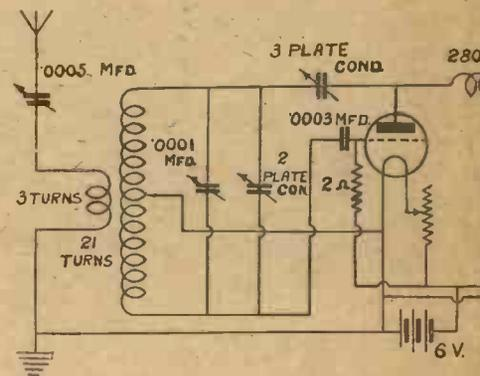
it will increase the capacity of the coil. An ultra efficient coil would be self-supporting. This has the disadvantage of being very sensitive to vibration, etc. Four thin strips of dry wood were used to support the turns. Here again ebonite could be used, but it would increase the capacity of the coil, the specific inductive capacity of ebonite being considerably larger than that of wood. Twenty-one holes,  $\frac{3}{16}$
