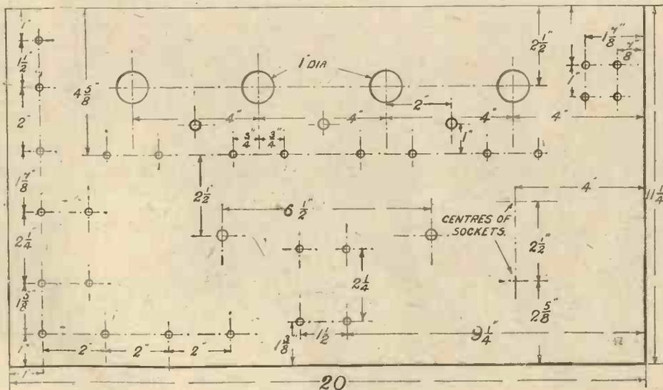
Fig. 2.—Drilling Plan of Panel.
