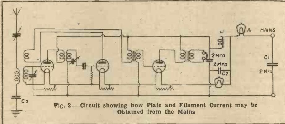
Fig. 2.—Circuit showing how Plate and Filament Current may be Obtained from the Mains
