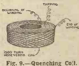
Fig. 9.—Quenching Coil.
