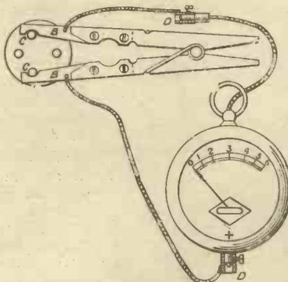
Testing Filament Voltage.
