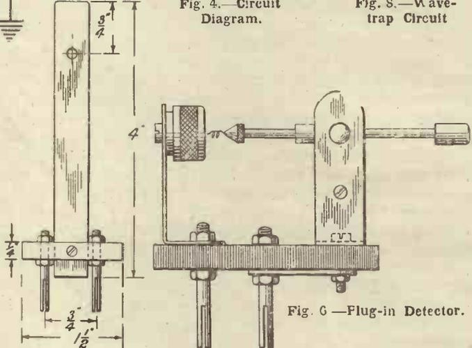
Fig. 6.—Plug-in Detector.
