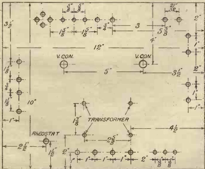
Fig. 1.—Drilling Plan of Panel.
