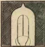
THE arched filament of the Wuncell Valve is further strengthened by means of a special centre support. Thus all possibility of sagging—no matter in which position the Valve is used—is entirely eliminated.
