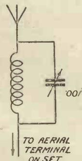
Fig. 5 (right).—Wave-trap Circuit.
