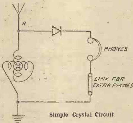
When only one pair of phones is in use the unused terminals are shorted by a metal strip or piece of copper wire. When it is desired to use both pairs of phones this shorting strip is removed and the phones substituted.—J. F. J.
