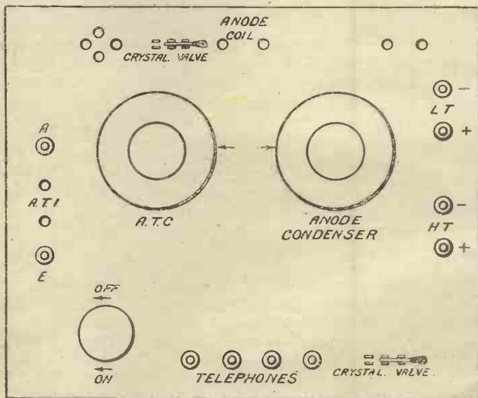
Fig. 2.—Layout of Panel.
