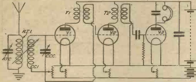
Fig. 2.—Circuit with Two Stages of H.F. Amplification.
