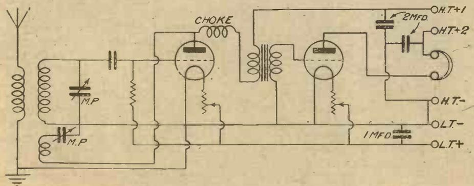
Fig. 1.—The First Experimental Circuit.
