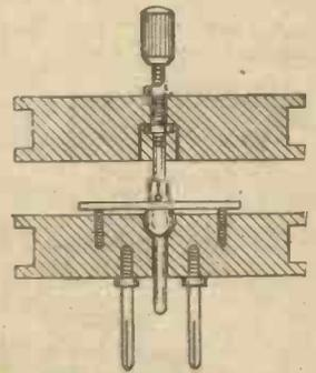
Simple Reaction Coupling Device.
