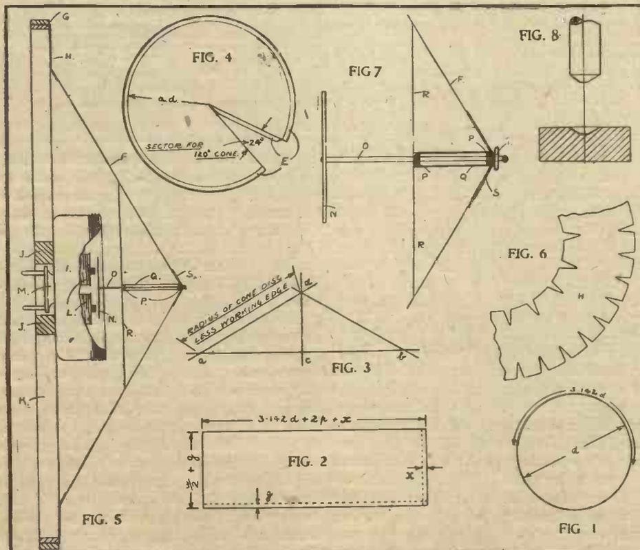
Fig. 1.—Relation between Diameter and Circumference of a Circle. Fig. 2.—Pattern for Pleated Strip. Fig. 3.—Method of Determining Radius of Disc for Cone. Fig. 4.—Pattern for Disc of Cone. Fig. 5.—Section of Cone Loud-speaker. Fig. 6.—Detail of "Flexible" Edge. Fig. 7.—Detail of Diaphragm Adjusting Device. Fig. 8.—Tool for Making Metal Nose.
