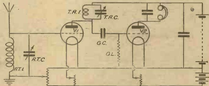
Fig. 1.—Typical Circuit with H.F. Amplification.
