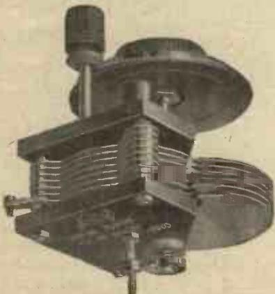
The Variable Condenser is truly a low loss model, with a very low minimum capacity, is of the straight line wavelength type, and each has a direct reading vernier movement. Compare the prices.
