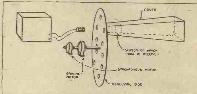
Diagrammatic Representations of the Baird Transmitter and Receiver.
