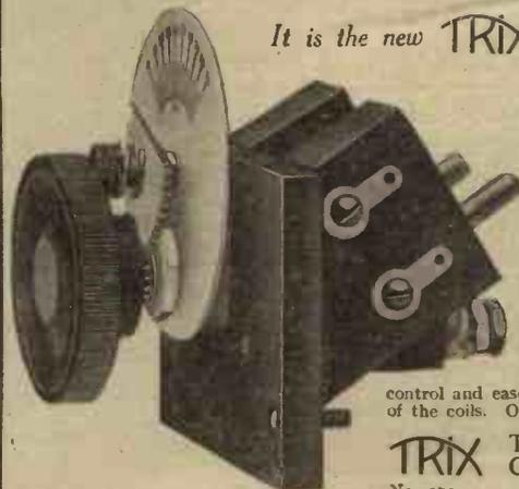
The moving coil holder moves at one quarter the speed of the control knob so that the movement is slow enough for very fine adjustment, while at the same time only one complete turn of the knob is needed to give the full range of movement when making a coarse setting.
