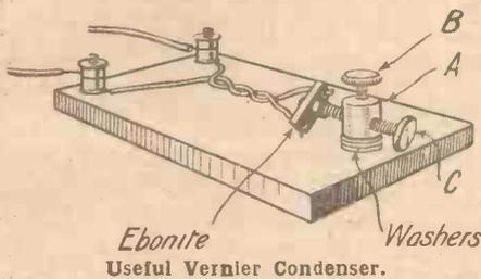
length by 2 in. in width. In one end of this mount a large terminal of the telephone or "push-in" type (A in the drawing), and in the opposite end place two terminals of any type.
