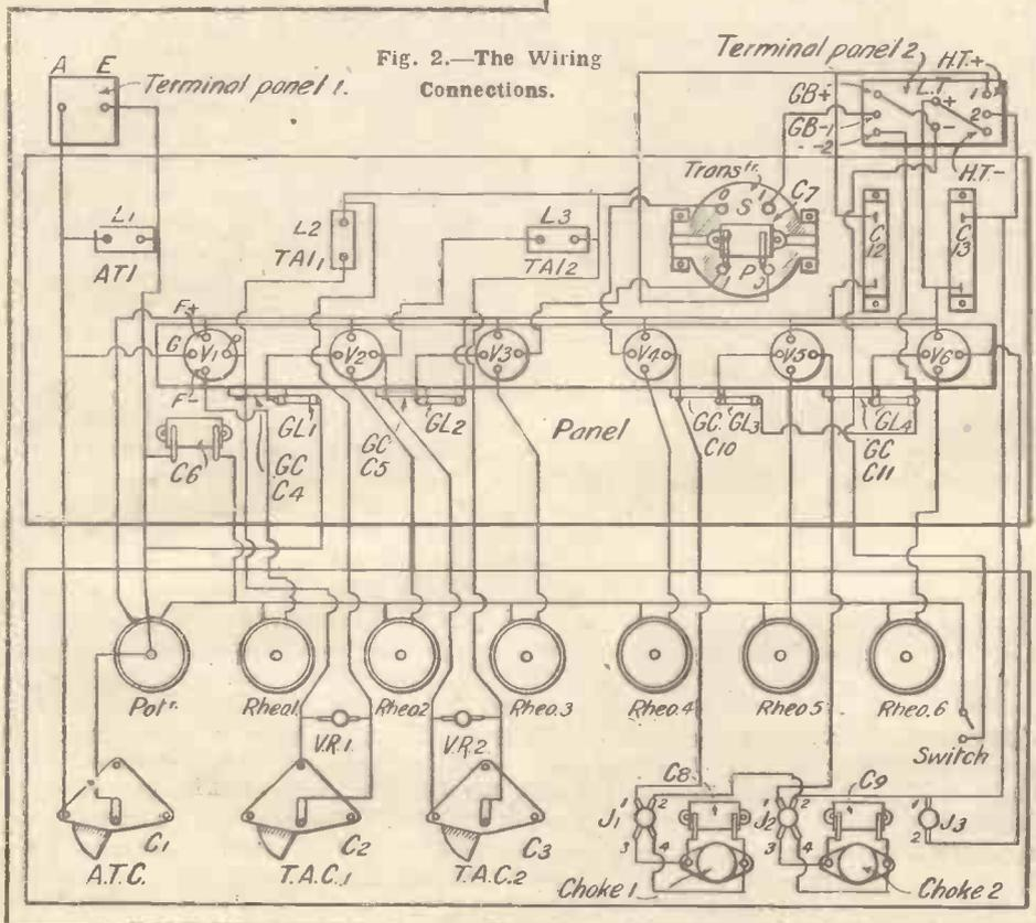
Fig. 2.—The Wiring Connections.
