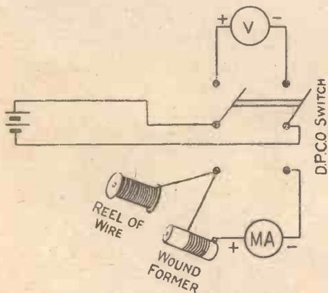
Fig. 4.—Testing the Resistance.
