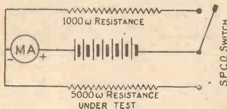
Fig. 5.—Testing the 5,000-ohm Resistance.
