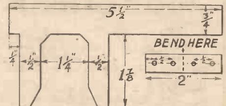
Fig. 5.—The Coil Support.
