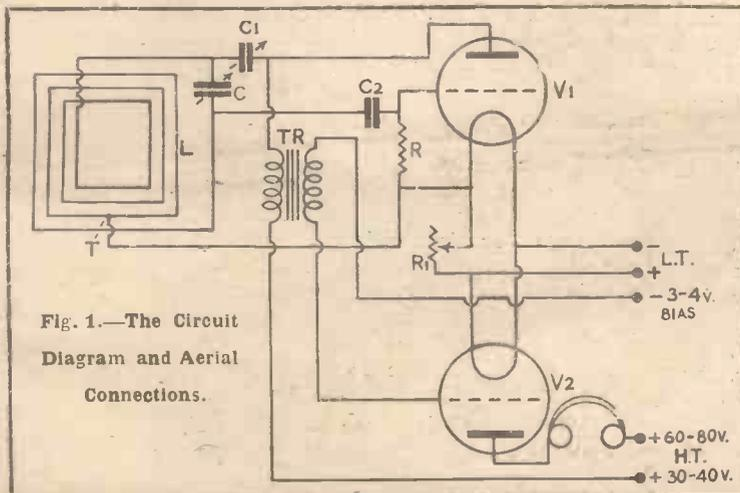
Fig. 1.—The Circuit Diagram and Aerial Connections.
