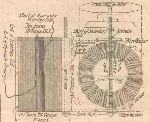
Fig. 2.—Details of Variocoupler.
