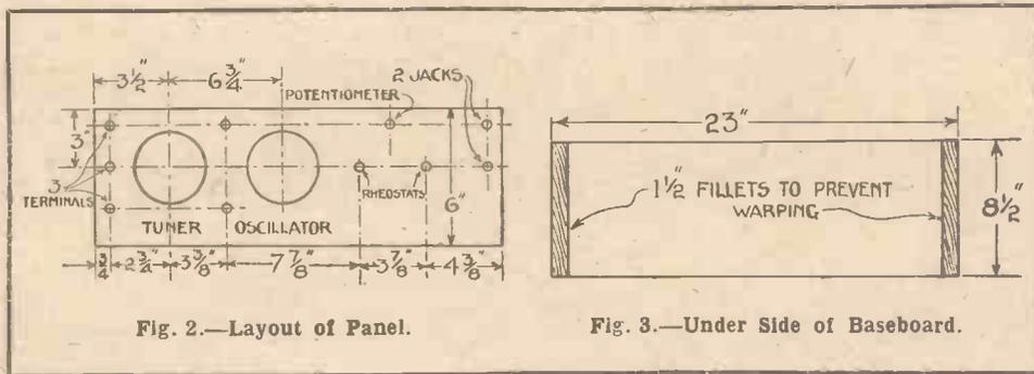
Fig. 2.—Layout of Panel.
