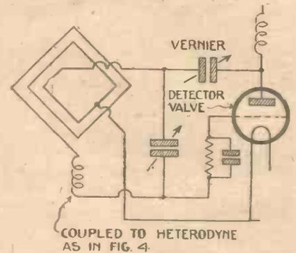
Fig. 10.—Capacity-reaction Coupling.
