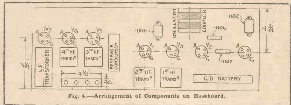
Fig. 4.—Arrangement of Components on Baseboard.
