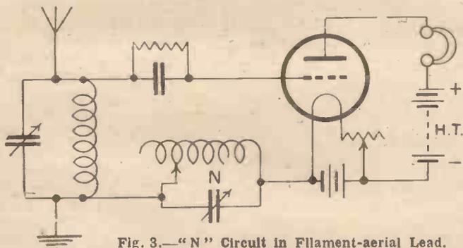
Fig. 3.—"N" Circuit in Filament-aerial Lead.
