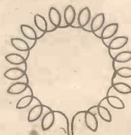
Fig. 3.—Diagram of Toroidal Coil.
