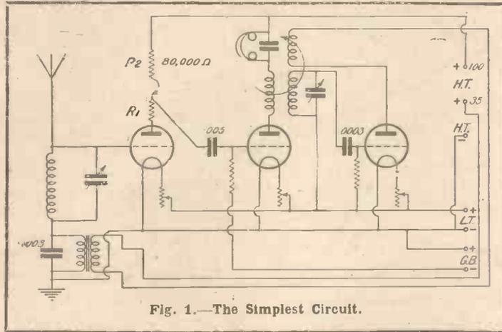
Fig. 1.—The Simplest Circuit.
