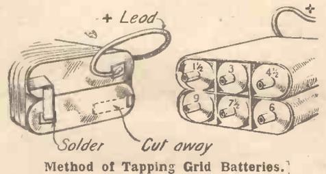
Method of Tapping Grid Batteries.
