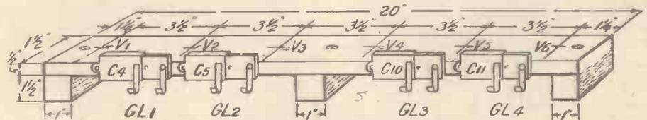
Fig. 5.—Details of Valve Bridge.
