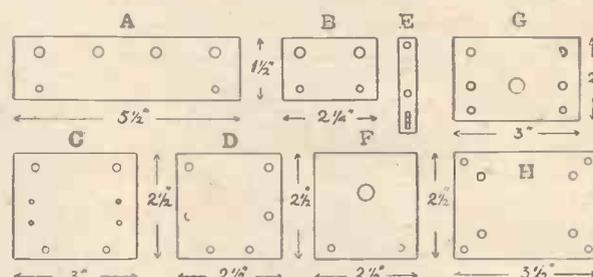
Fig. 5.—Details of Sub-panels.
