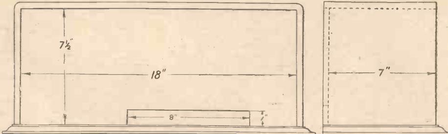
Fig. 2.—Constructional Details of Cabinet.
