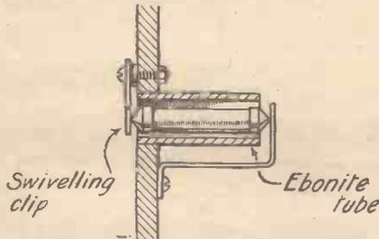
Details of Grid Leak Mounting.
