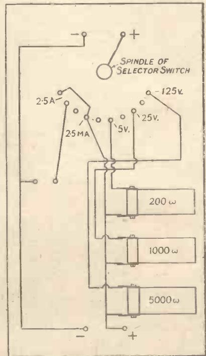
Fig. 10.—Connections for Instrument.
