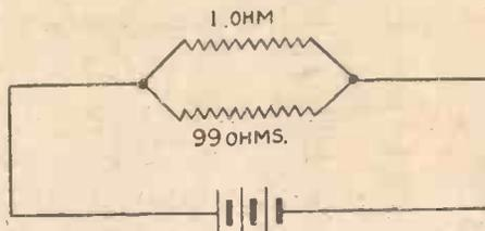
Fig. 1.—Explanation of Shunt Circuit.
