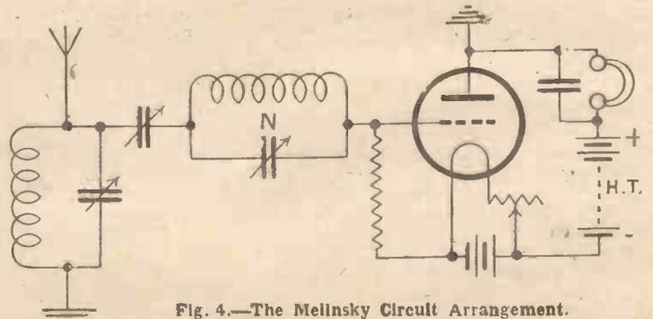
Fig. 4.—The Melnsky Circuit Arrangement.
