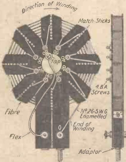
Fig. 2.—Constructional Details of Coil
