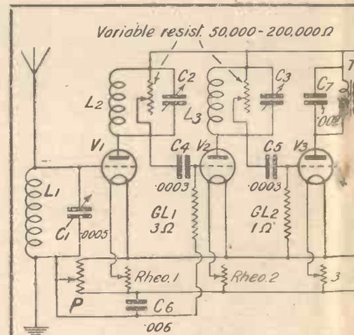
Fig. 1.—Theoretical Circuit of the Receiver
