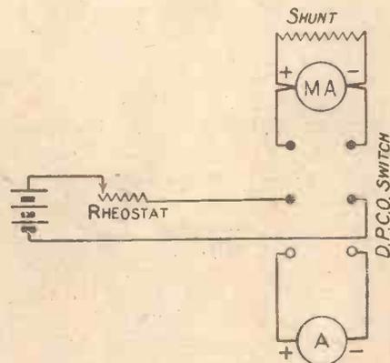
Fig. 6.—Circuit for Testing Shunt.
