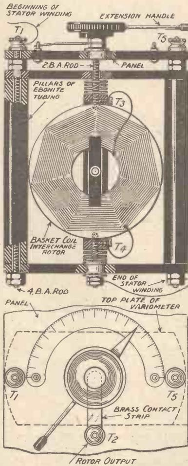
Fig. 1.—Elevation and Plan of Variometer Tuner.
