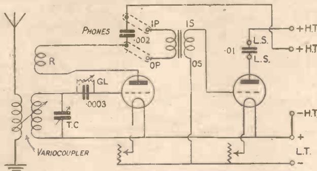
Fig. 1.—The Circuit Diagram.
