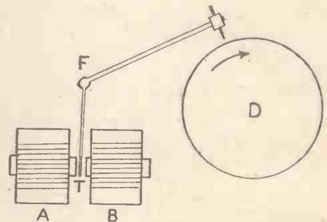
Fig. 3.—Diagram of Jenkins' Receiving Apparatus.
