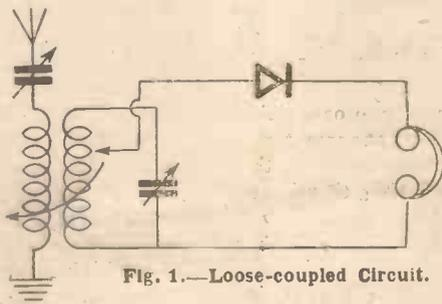
Fig. 1.—Loose-coupled Circuit.
