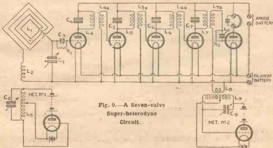
Fig. 9.—A Seven-valve Super-heterodyne Circuit.
