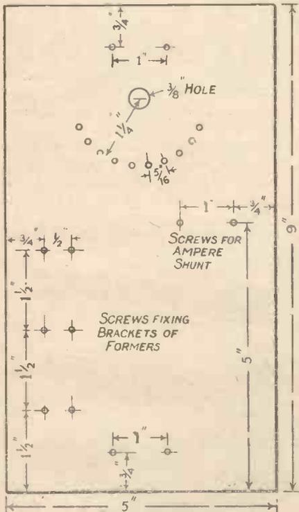
Fig. 9.—Panel-drilling Diagram.
