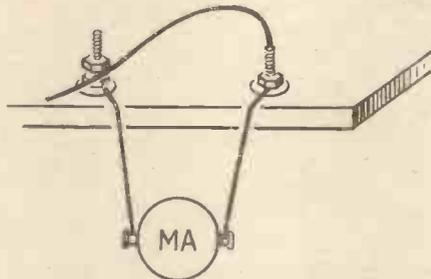
Fig. 8.—Adjusting the Ammeter Shunt.
