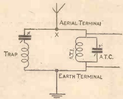
Fig. 2.—An Effective Wave-trap Arrangement.
