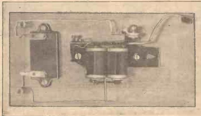
Photograph of Overload Indicator for the H.T. Circuit.
