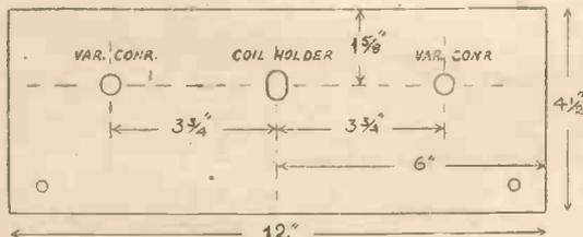
Fig. 1.—Layout of Panel.
