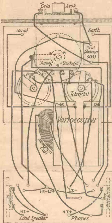
Fig. 5.—Developed Wiring Diagram.
