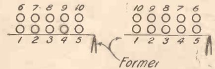
Windings of High-capacity Coils.
