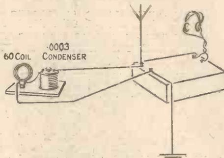
Fig. 3.—A "Hook-up" Wave-trap.
