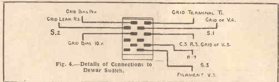
Fig. 4.—Details of Connections to Dewar Switch.
