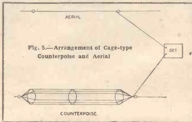
Fig. 5.—Arrangement of Cage-type Counterpoise and Aerial
