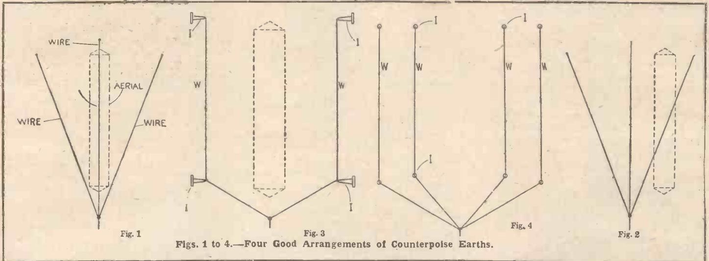
Figs. 1 to 4.—Four Good Arrangements of Counterpoise Earths.
