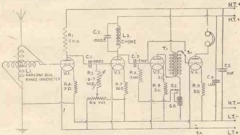
Fig. 1.—Circuit Diagram of One-dial Four-valver.
