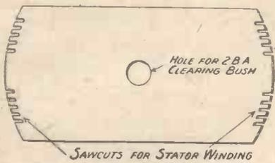
Fig. 2.—Shape of Stator Plates.
