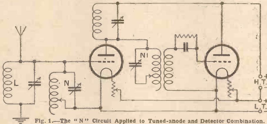
Fig. 1.—The "N" Circuit Applied to Tuned-anode and Detector Combination.
