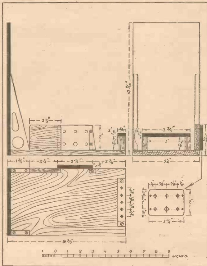
Fig. 3.—Details of Baseboard and Panel.
