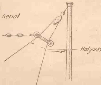
Arrangement of Halyards and Pulleys.
