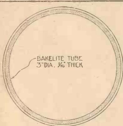
Fig. 5.—Single-layer solenoid, wound with No. 22 d.s.c. wire. Length of winding, 1½ in. Inductance, 153 microhenries. H.F. resistance at 400 m. = 5.2 ohms. Figure of merit, 29.5.
