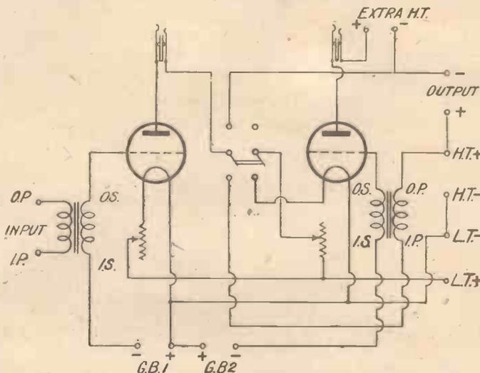
Fig. 2.—Circuit Diagram of Power Amplifier.
