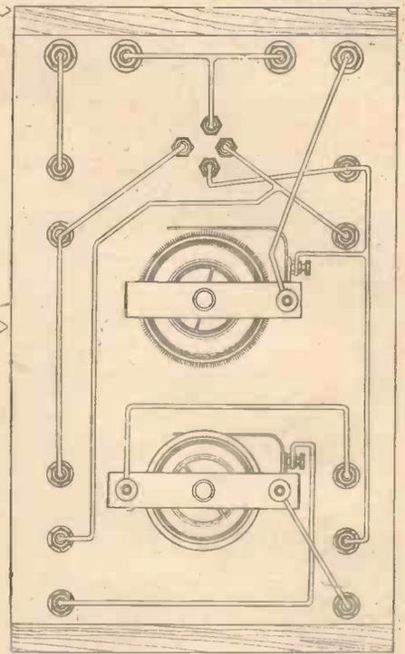
Fig. 3.—Connections on Back of Panel.
