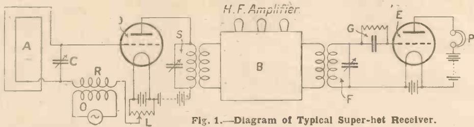
Fig. 1.—Diagram of Typical Super-hot Receiver.
