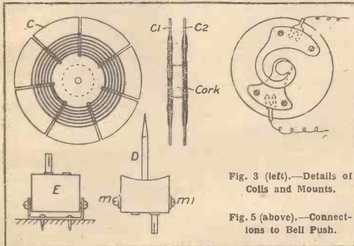
Fig. 3 (left).—Details of Coils and Mounts.
