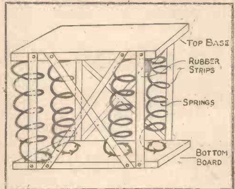
Fig. 2.—Construction of Anti-vibration Base.
