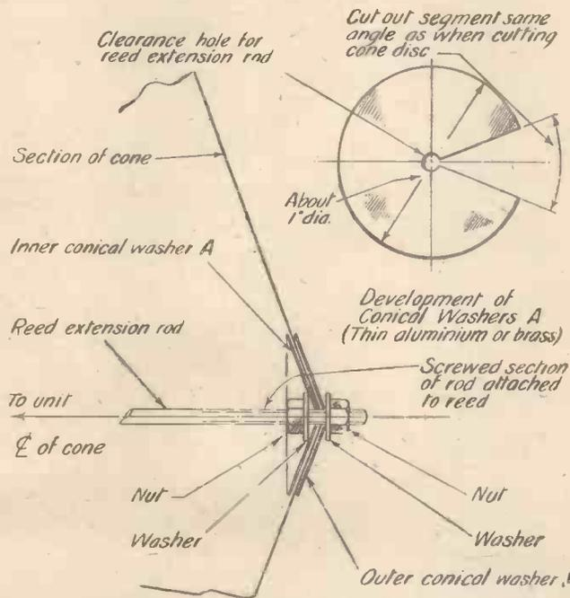
Diagrams showing how the Cone is Built Up.
