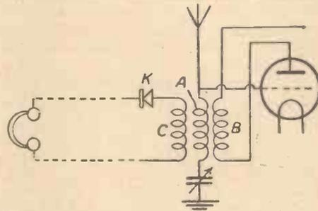
Fig. 1.—Circuit Diagram of Coupled Receiver.
