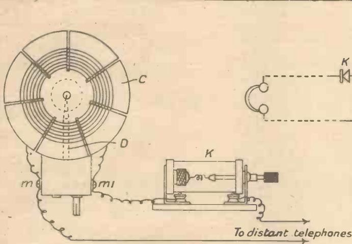
Fig. 4.—Connections of Coil and Detector.
