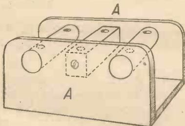
Fig. 2.—Adjustable Coil Holder.
