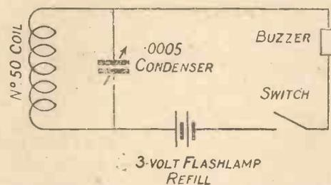
Circuit Diagram of Substitute for Wavemeter.
