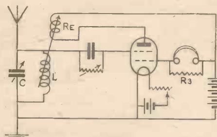
Fig. 7.—Circuit with Magnetic Reaction.
