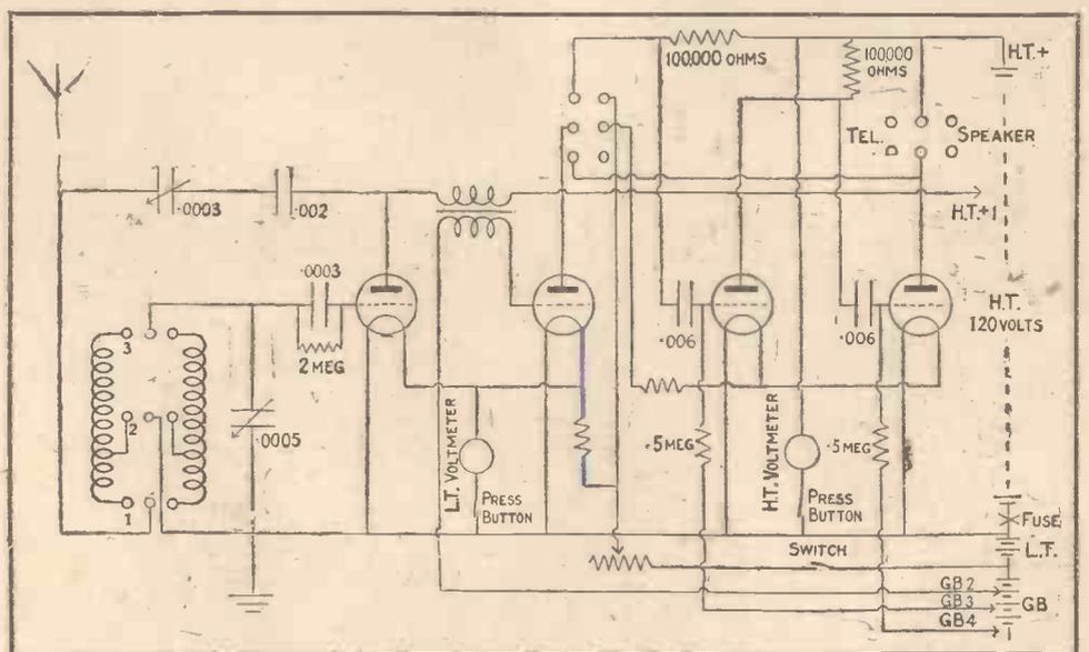
second valve. The other connections to the transformer are by flex, so that they may be readily altered. One length of flex from the opposite end of the secondary coil passes along the back edge of the baseboard so as to cross to the grid bias battery.
