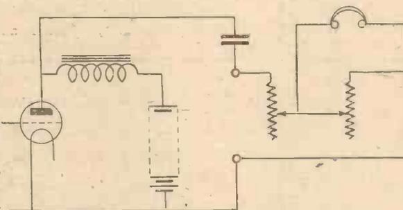
Fig. 8.—Another Scheme of Connections for the Audibility Meter.
