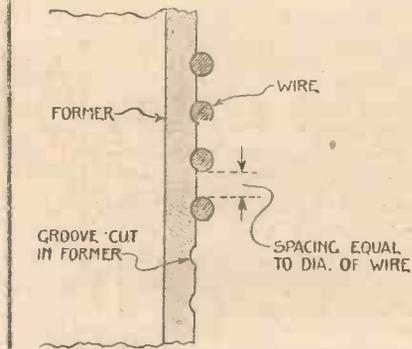
Fig. 12.—Method of Spacing Turns of Metaloid Coil.
