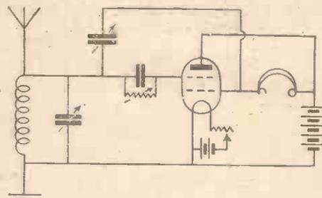
Fig. 8.—Circuit with Capacity Reaction.
