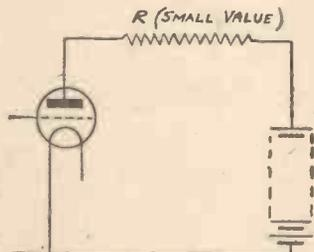
Fig. 3.—Anode Circuit with Resistance.
