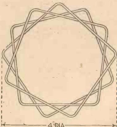
Fig. 3.—Cylindrical basket-weave coil, wound with No. 18 d.c.c. wire. Length of winding, 1½ in. Inductance, 182 microhenries. H.F. resistance at 400 m. = 4.5 ohms. Figure of merit, 40.5.
