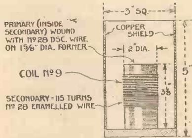
Fig. 11.—Metaloid coil in sectional elevation. Inductance of secondary, 320 microhenries. Resistance (average), 9.5 ohms. Figure of merit, 33.7.
