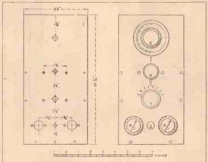
Fig. 2.—Layout and Plan of Panel.
