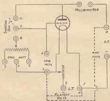
Fig. 4.—Diagram of Connections.
