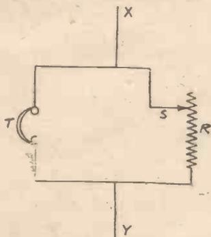
Fig. 1.—Phone Circuit with Resistance.
