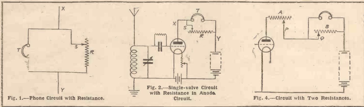
Fig. 1.—Phone Circuit with Resistance.
