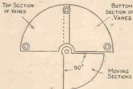
Fig. 9.—Diagram of Compensator Condenser.
