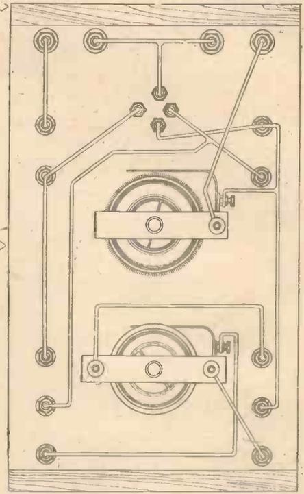
Fig. 3.—Connections on Back of Panel.
