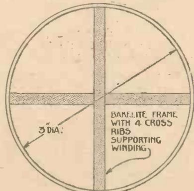
Fig. 2.—Single-layer solenoid, wound with No. 22 d.c.c. wire. Length of winding, 2½ in. Inductance 246 microhenries. H.F. resistance at 400 m. = 5.7 ohms. Figure of merit, 43.
