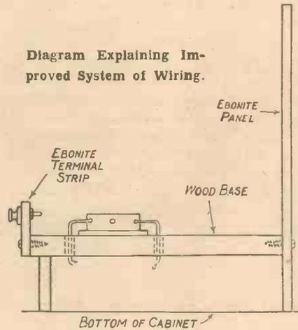
ciency owing to induction, the following method is suggested: That is, the wood baseboard be lifted about 1 in. from the foot of the ebonite panel and secured in
