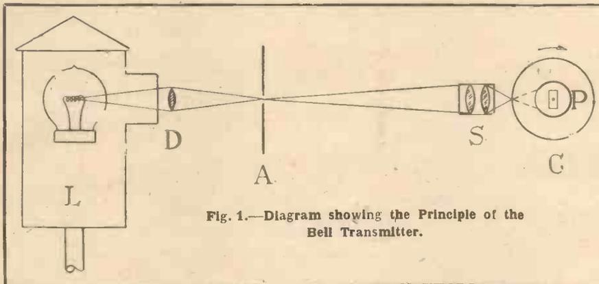
Fig. 1.—Diagram showing the Principle of the Bell Transmitter.
