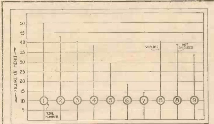
Fig. 10.—Comparison of Low-loss Coils.
