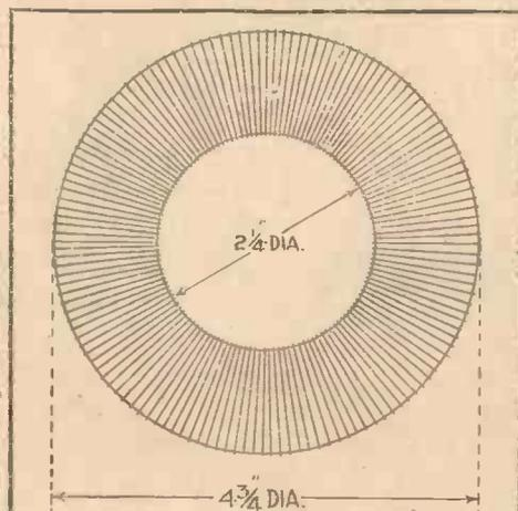
Fig. 6.—Toroid coil, wound with No. 20 d.c.c. wire, supported by Bakelite frame. Inductance, 120 microhenries. H.F. resistance at 400 m. = 9.8 ohms. Figure of merit, 13.4.
