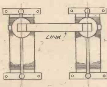
Figs. 5 and 6.—Methods of Coupling Pairs of Resistances.
