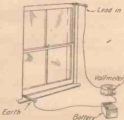
Method of Testing Aerial Insulation.
