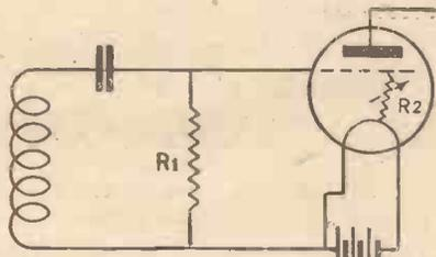
Fig. 1.—Diagram showing how the Grid Leak Functions.
