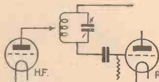
Fig. 4.—Tuned-anode Coupling.
