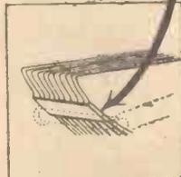
Fixed and moving plates are of brass, riveted together and soldered, ensuring permanent alignment and sound electrical connection.
