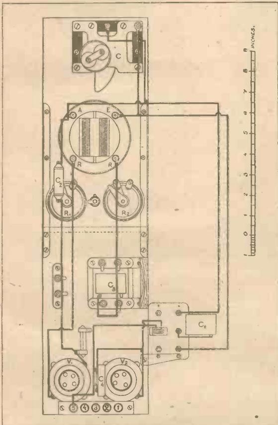
Fig. 5.—Diagram of Second Stage of Wiring.
