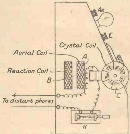
Fig. 2.—Suggested Arrangement of Coupling Coils.
