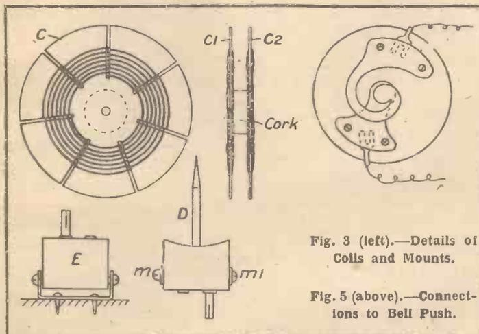
Fig. 3 (left).—Details of Coils and Mounts.
