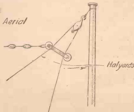
Arrangement of Halyards and Pulleys.
