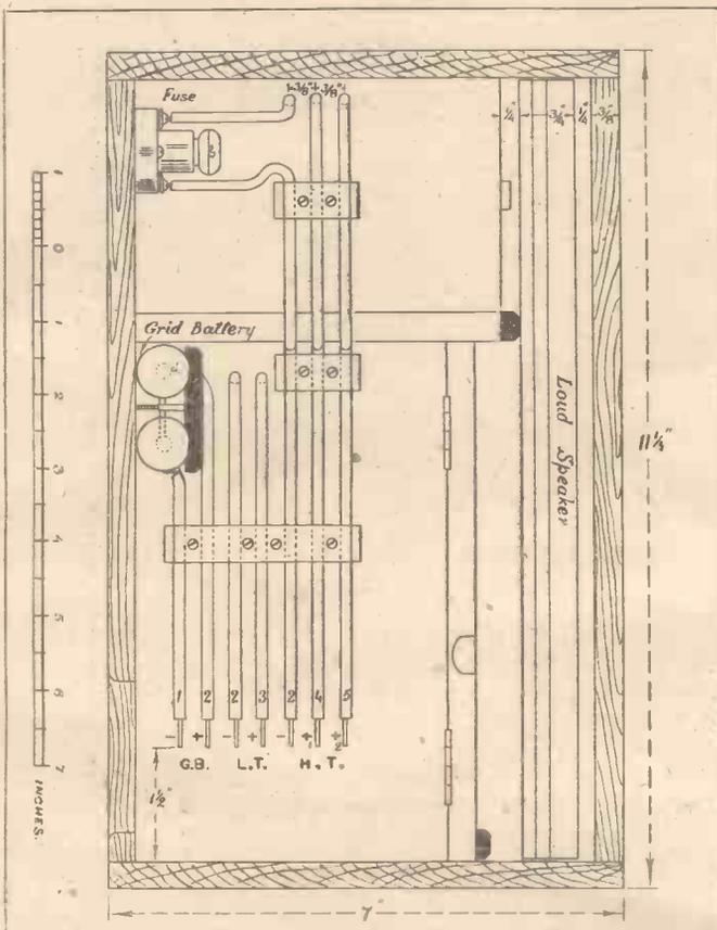
Fig. 9.—Section showing Construction of Cabinet.
