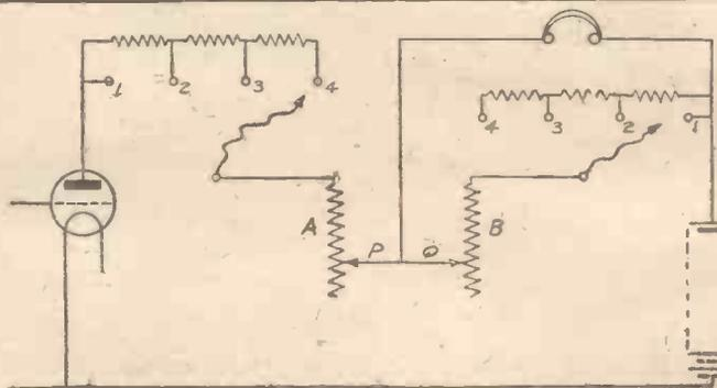
Fig. 7.—Connections for Audibility Meter.
