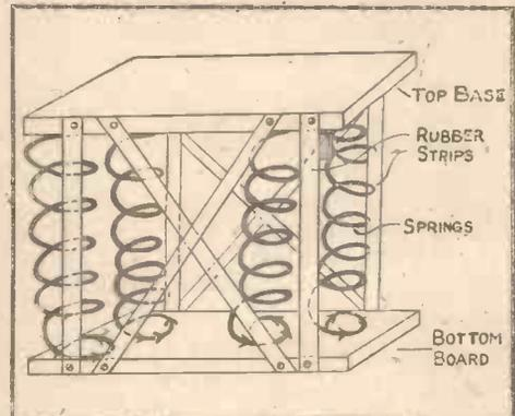
Fig. 2.—Construction of Anti-vibration Base.
