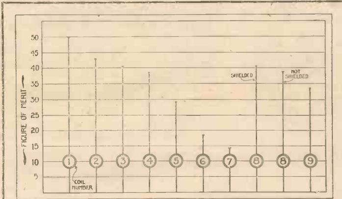
Fig. 10.—Comparison of Low-loss Coils.
