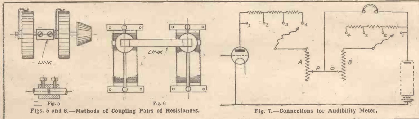
Figs. 5 and 6.—Methods of Coupling Pairs of Resistances.
