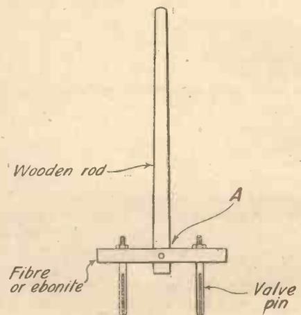
Fig. 3.—Support for Coil.
