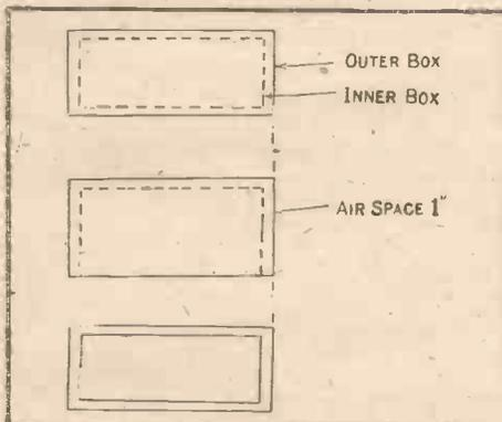
Fig. 1.—Construction of Sound-proof Box.
