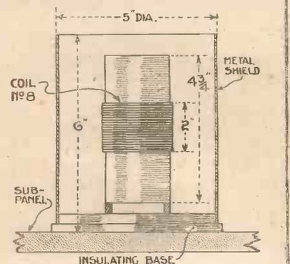
Fig. 9.—Details of Walbert Shielded Coil.
