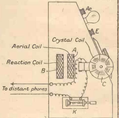
Fig. 2.—Suggested Arrangement of Coupling Coils.
