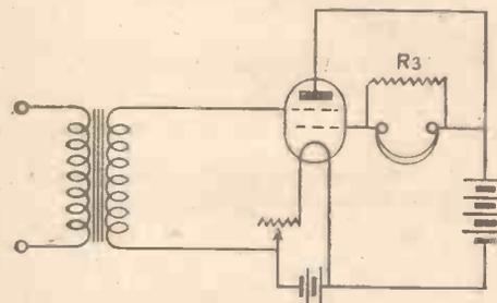
Fig. 11.—L.F. Circuit with Two-grid Valve.
