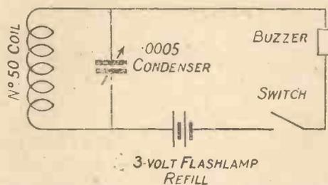
Circuit Diagram of Substitute for Wavemeter.
