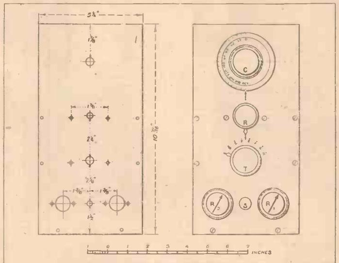
Fig. 2.—Layout and Plan of Panel.
