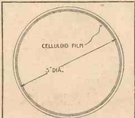
Fig. 1.—Single-layer solenoid, wound with No. 22 s.s.c. wire, spaced half diameter of wire. Length of winding, 2½ in. Inductance, 276 microhenries. H.F. resistance at 400 m. = 5.5 ohms. Figure of merit, 50.
