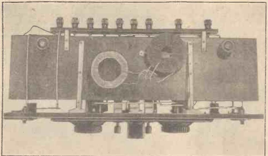
Under-side View showing Tuning Coils.
