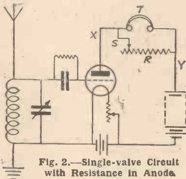
Fig. 2.—Single-valve Circuit with Resistance in Anode Circuit.
