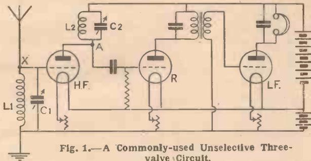
Fig. 1.—A Commonly-used Unselective Three-valve Circuit.
