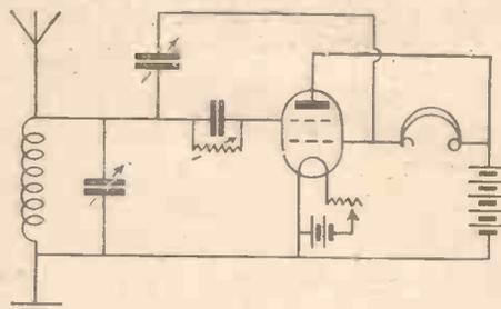
Fig. 8.—Circuit with Capacity Reaction.
