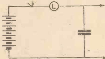
Method of Checking Leakage.
