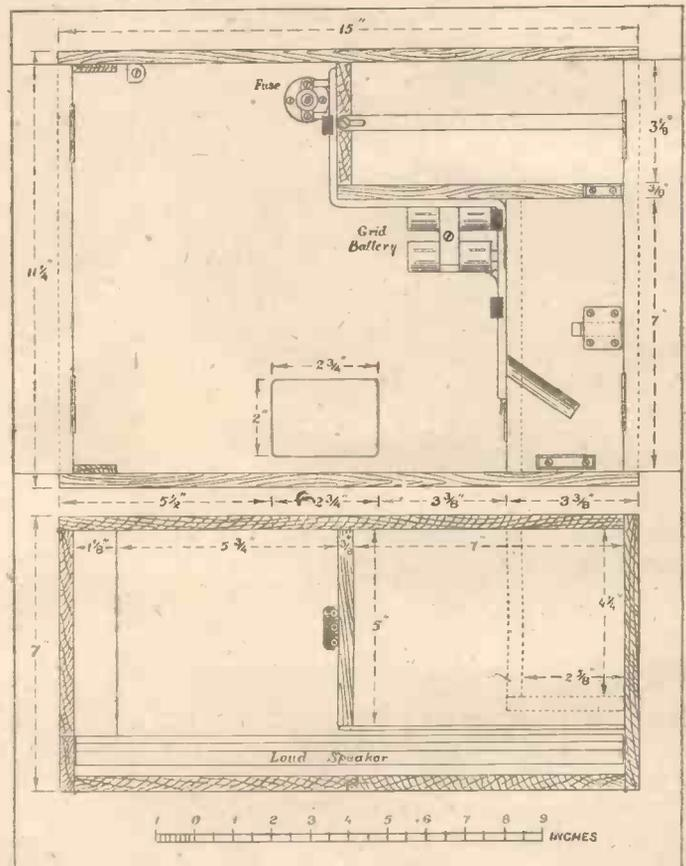
Fig. 10.—Elevation and Cross Section of Cabinet.
