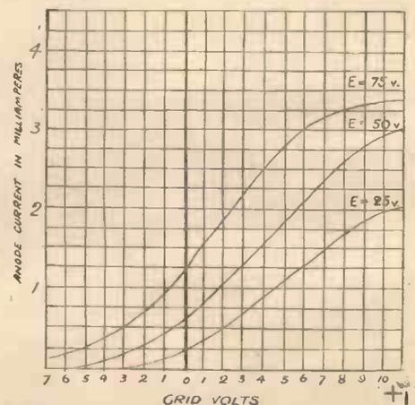
Fig. 1.—Example of Characteristic Curve.
