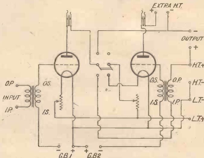
Fig. 2.—Circuit Diagram of Power Amplifier.
