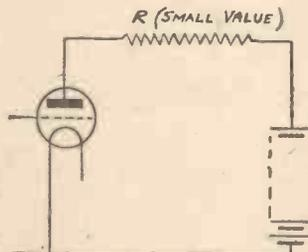
Fig. 3.—Anode Circuit with Resistance.
