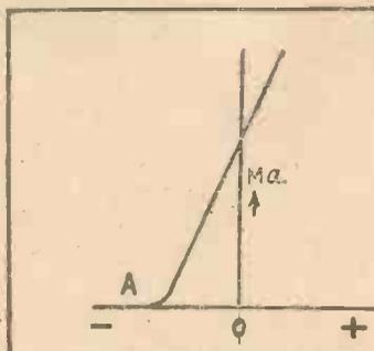
Fig. 4.—Curve showing Working Point of Valve  $V_1$ .
