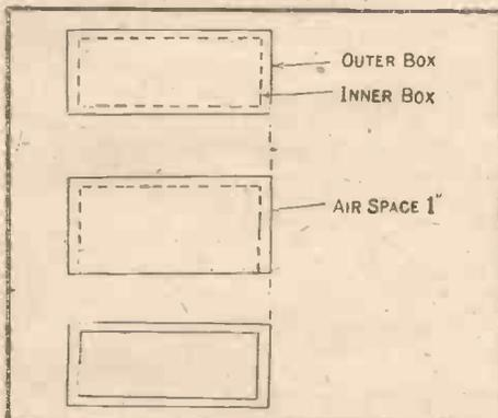
Fig. 1.—Construction of Sound-proof Box.
