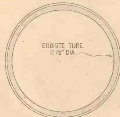
Fig. 8.—Walbert coil, wound 50 turns per inch. Length of winding, 2 in. Figure of merit (not shielded), 38.5. Figure of merit (shielded), 40.5.
