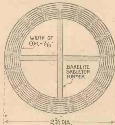
Fig. 7.—Multi-layer honeycomb coil, wound with No. 24 d.s.c. wire. Inductance, 320 microhenries. H.F. resistance at 400 m. = 22.5 ohms. Figure of merit, 14.2.
