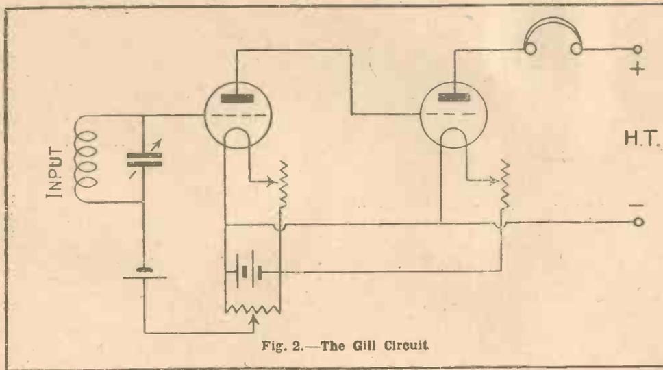
Fig. 2.—The Gill Circuit
