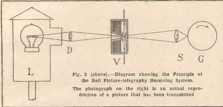
Fig. 3 (above).—Diagram showing the Principle of the Bell Picture-telegraphy Receiving System.
