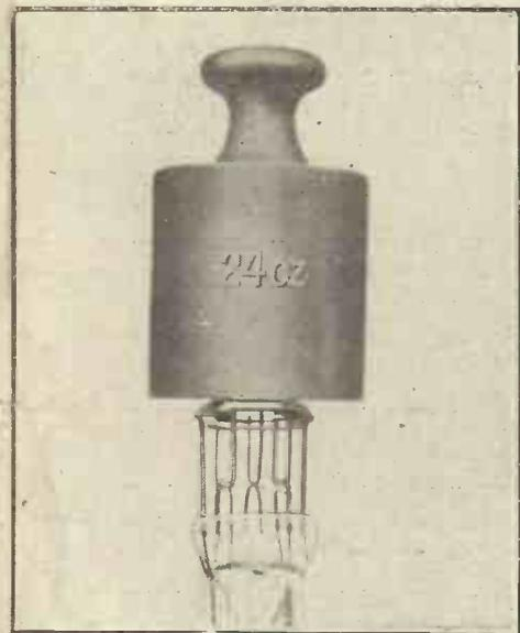
Fig. 5.—An Experiment in which the Anode of a P.M. Valve Sustained a Pressure of 24 oz.
