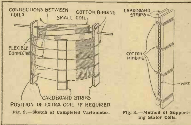
Fig. 2.—Sketch of Completed Variometer.
