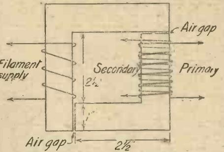
Fig. 1.—Details of Transformer Coil.
