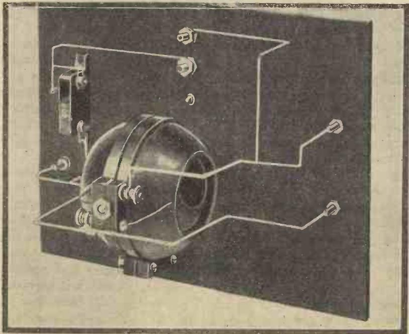
Back-of-panel View of Variometer-tuned Crystal Set.
