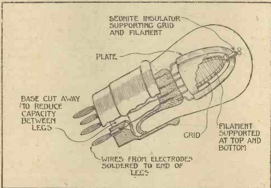
Most valves have cylindrical grids and plates; the above Valve (Cossor) is an example with hood-shaped grid and plate.
