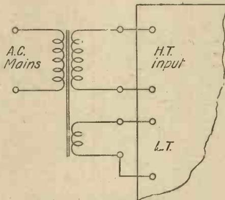
Fig. 2.—Connections of Transformer.
