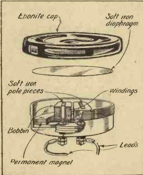
The Construction of a Phone Ear-piece
