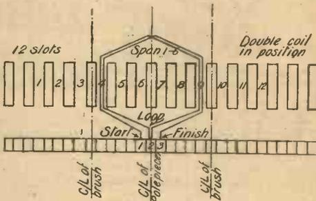
Diagram of 12-slot Armature and 24-part Commutator.
