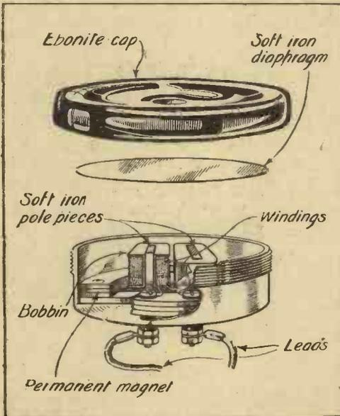
The Construction of a Phone Ear-piece
