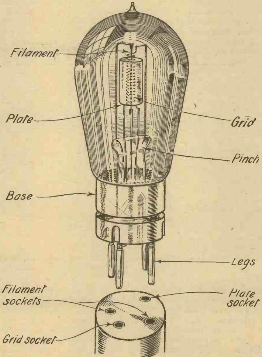
This illustration shows the construction of a typical valve. The filament, grid, and plate are supported clear of each other within the glass bulb, from which all air is withdrawn. Leads from the three electrodes are taken through the "pinch" to the unevenly-spaced legs.
