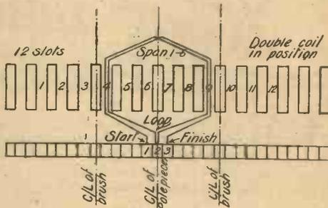
Diagram of 12-slot Armature and 24-part Commutator.
