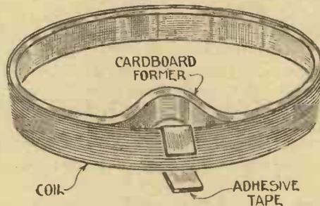
Fig. 1.—Method of Making Rotor Coil.
