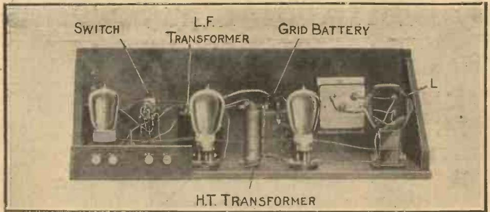
Back View of Receiver showing Disposition of Components.
