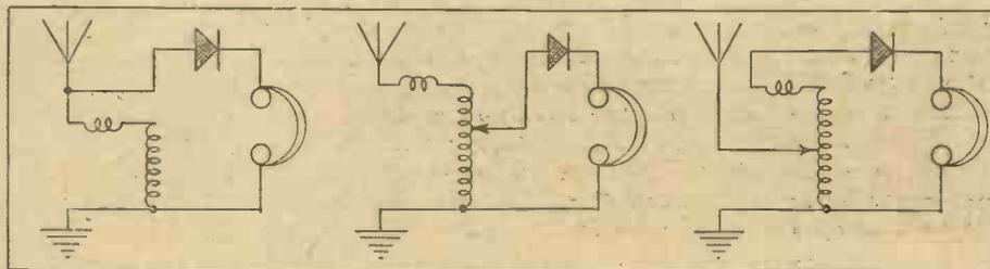
Figs. 4, 5 and 6.—Suggested Circuits for the Receiver.
