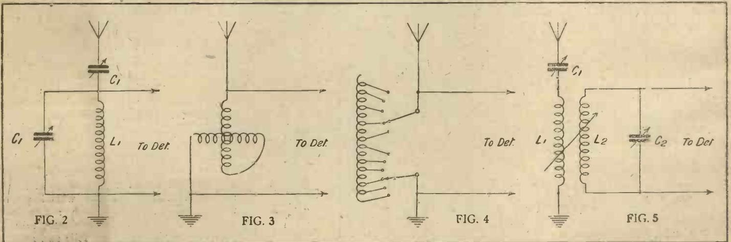
Figs. 2, 3 and 4.—Selective Circuits Employing Low-loss Coils.
