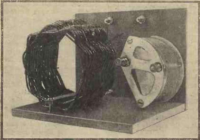
Interior of Crystal Set tuned by Coil and Variable Condenser.
