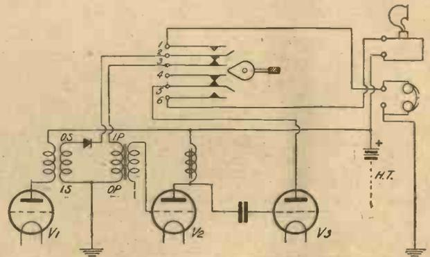
Fig. 3.—Circuit Diagram of Telephone side of Switch.
