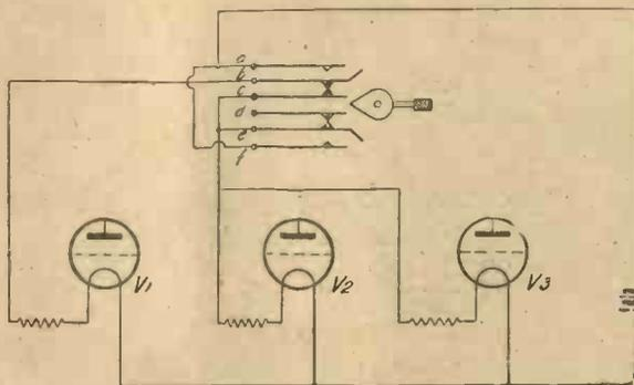
Fig. 2.—Circuit Diagram of Filament Section of Switch.
