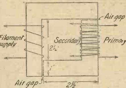
Fig. 1.—Details of Transformer Coil.
