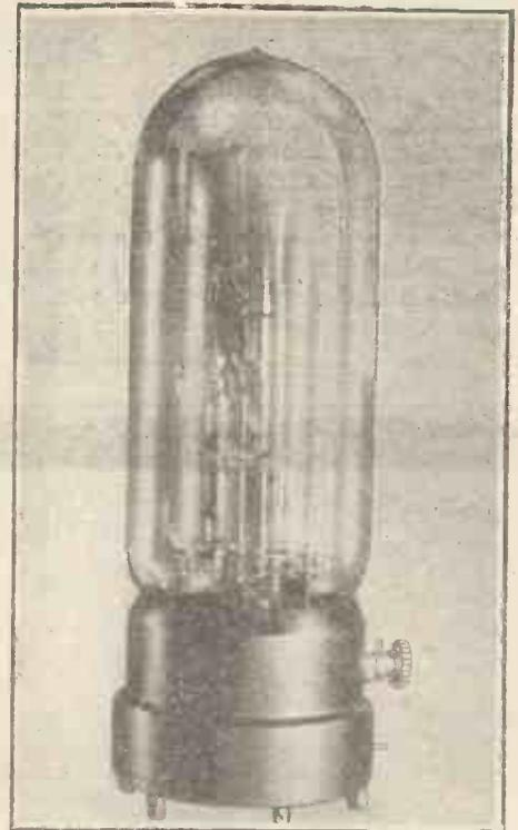
Fig. 6.—Triplex Valve of Special Design.
