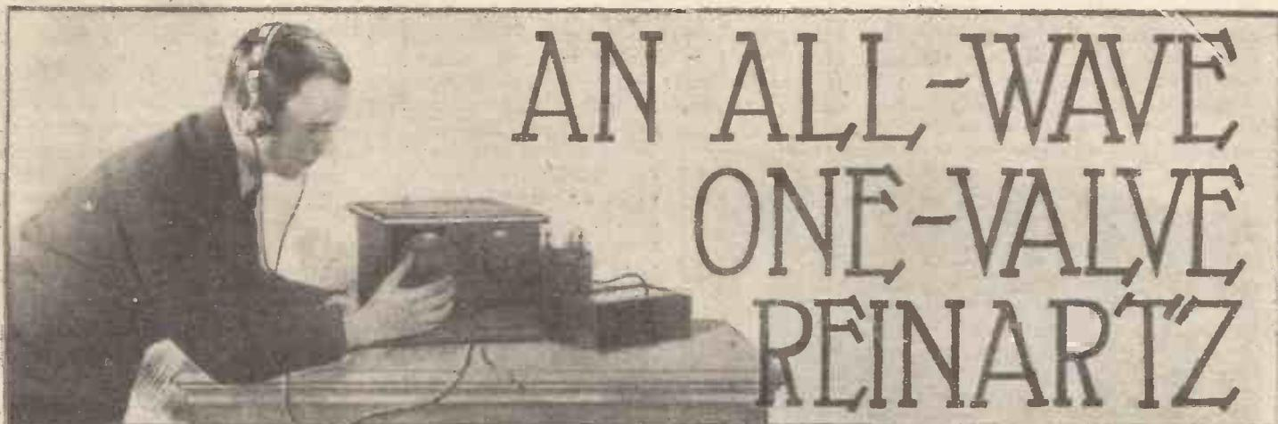
**C**APACITY-CONTROLLED magnetic reaction, familiarly known as Reinartz reaction, is fast becoming the most popular and widely-used system whereby a smooth and gradual application of reaction is obtained. The one-valve receiver shown in the photographs incorporates a well-tried and highly satisfactory form of Reinartz reaction.
