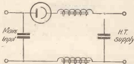
Fig. 14.—Smoothing Circuit with Osglim Lamp (see Fig. 14). An arrangement such as this will be found very useful where a relatively small H.T. current is desired and
