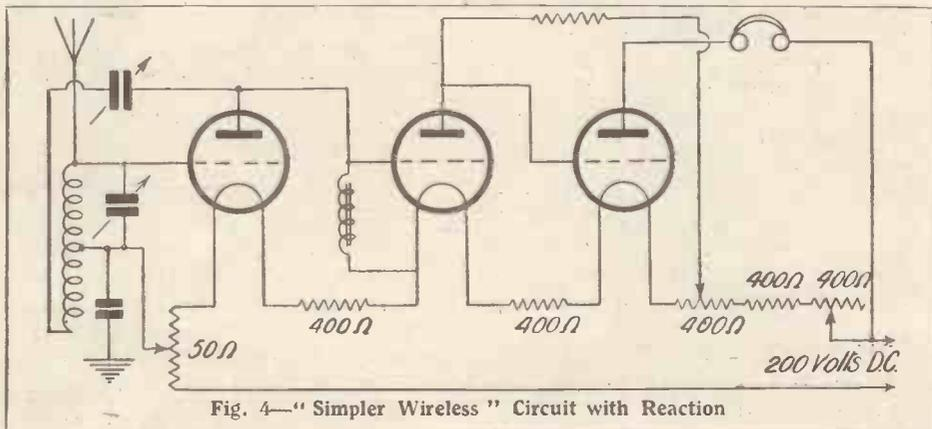
Fig. 4—"Simpler Wireless" Circuit with Reaction
