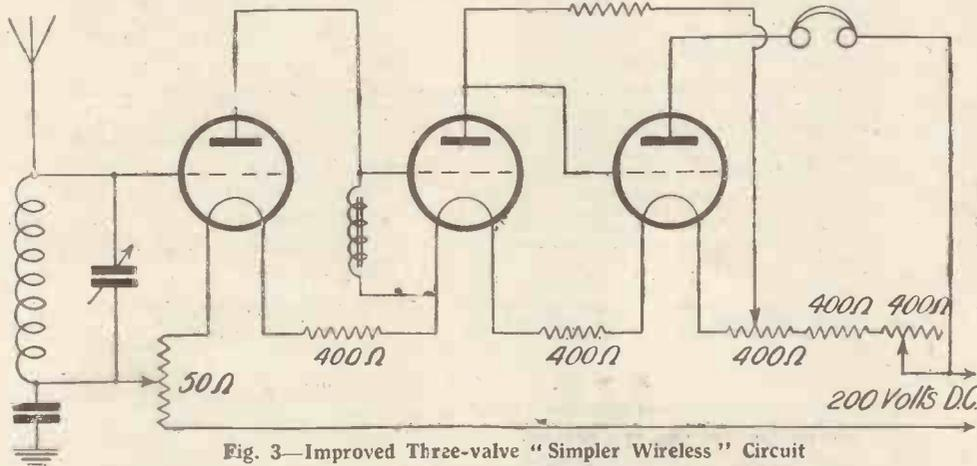
Fig. 3—Improved Three-valve "Simpler Wireless" Circuit
