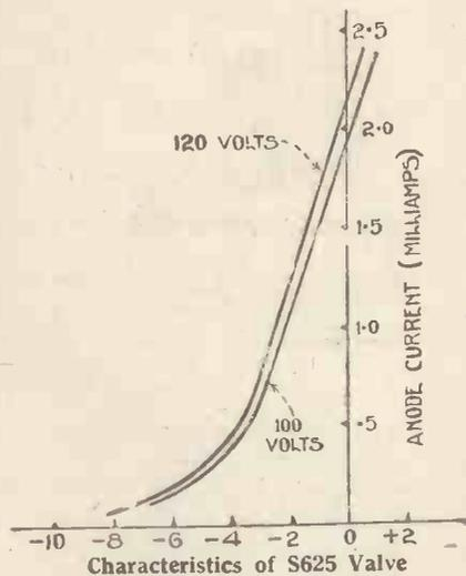
Now, an increase in the internal impedance of the valve is all to the good, as it obviates the valve damping, which is so commonly experienced in normal circuits. If the shunting effect of the valve on the tuned circuit is reduced the circuit is more sharply tuned. At the same time, the increase in the amplification factor enables us to use plain tuned-anode circuits without the necessity for a transformer, and still obtain a high amplification from the stage.
