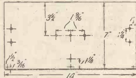
Drilling Diagram of Panel
