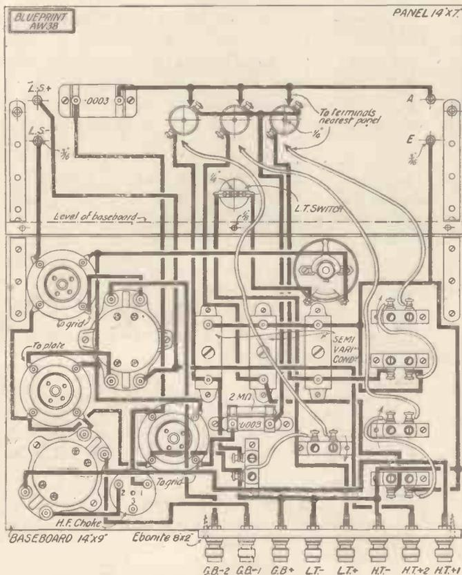
The Wiring Diagram
