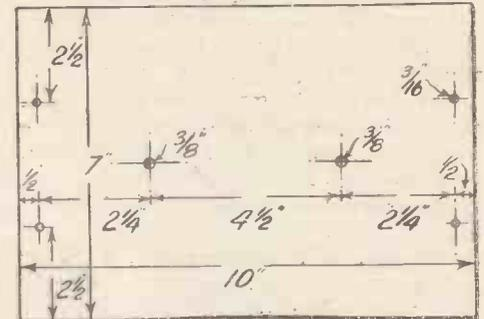
Drilling Diagram of Panel
