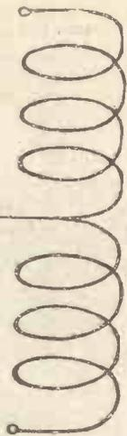
NOW that there are so many centre-tapped plug-in coils available, we can make more general use of circuits incorporating them. Many circuits can be more simply interpreted in a practical form by means of centre-tapped coils. Take, for example, the two-valve circuit shown by the accompanying theoretical diagram. It is the familiar Hartley reaction arrangement, whereby the tuning and reaction coils are combined in one centre-tapped plug-in coil.
