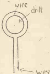
at the end of a piece of wire by bending it round a drill and pinching the ends together with a pair of pliers. The drill is chosen of such a size that the loop formed will just slip on to the screw. M. C.
