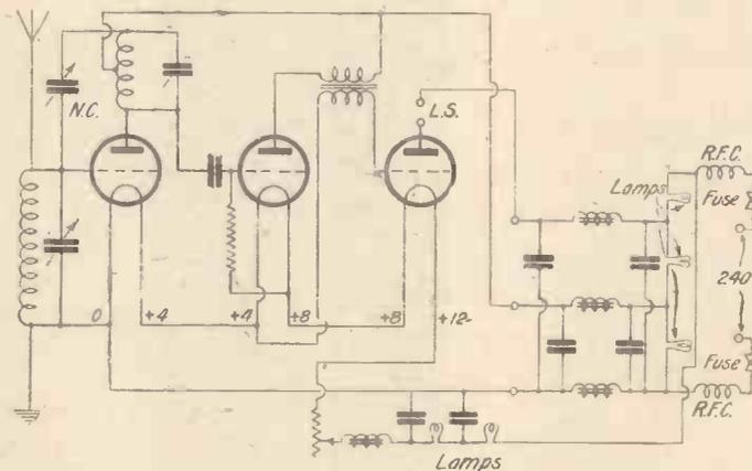
Fig. 19.—A Three-valve Mains Circuit
