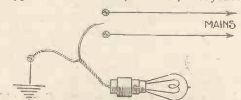
Fig. 3—Testing for Earthed Main
