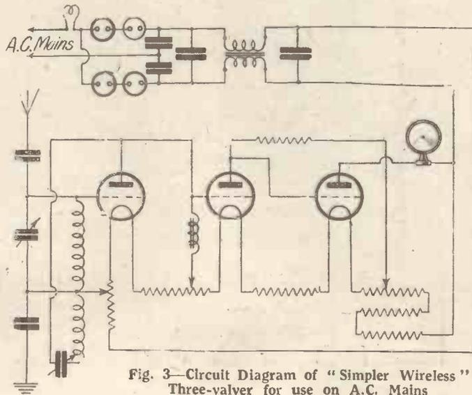
Fig. 3—Circuit Diagram of "Simpler Wireless" Three-valver for use on A.C. Mains
