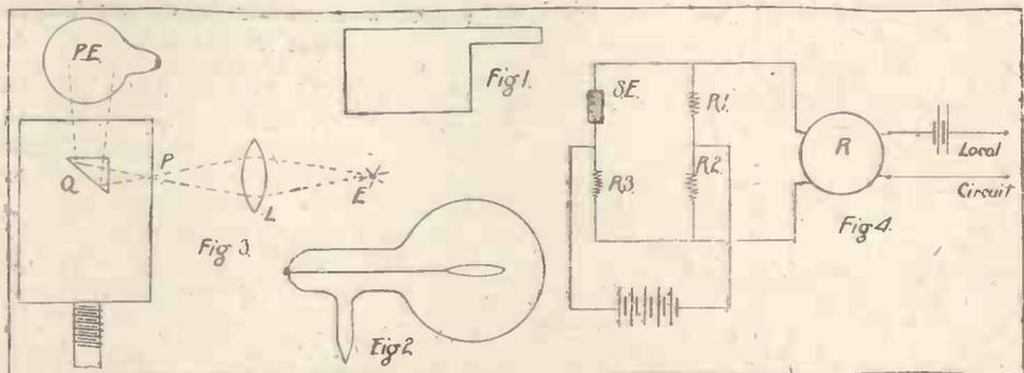
Fig. 1—A Simple Photo-electric Cell    Fig. 2—The Commercial Type of Photo-electric Cell
