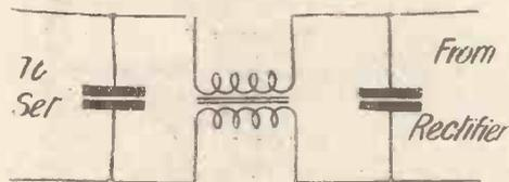
Fig. 2—The Simple Smoothing Arrangement
