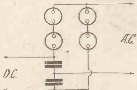
Fig. 1—How the Rectifier Cells are Connected
