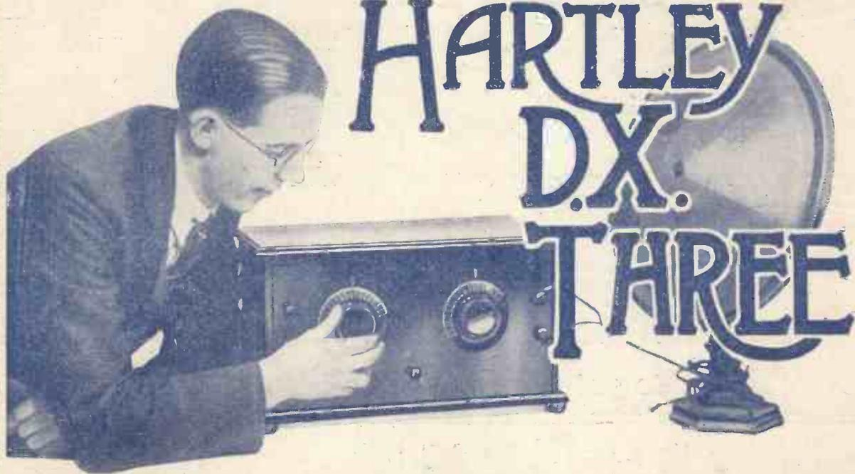
THE HARTLEY CIRCUIT EMBODIED GIVES SELECTIVE TUNING AND SMOOTH REACTION WITH A SINGLE CENTRE-TAPPED COIL. THE HIGH-QUALITY REPRODUCTION WILL STRONGLY APPEAL TO THE CRITICAL LISTENER.
