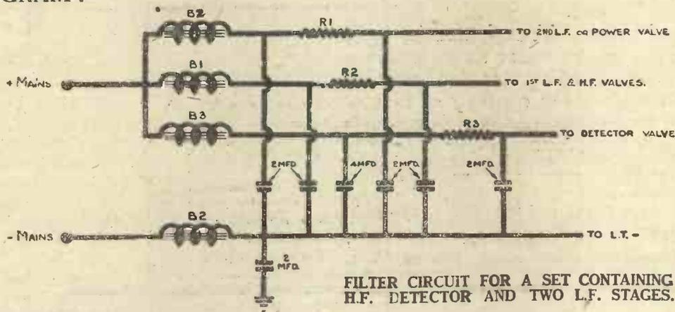
FILTER CIRCUIT FOR A SET CONTAINING H.F. DETECTOR AND TWO L.F. STAGES.
