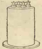
Marconiphone H.F. Choke. Inductance 100,000 microhenries resistance 700 ohms. Very efficient on wave-lengths up to 4,000 metres. 10/6.
