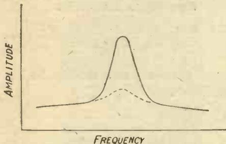
Diagram showing effect of damping
