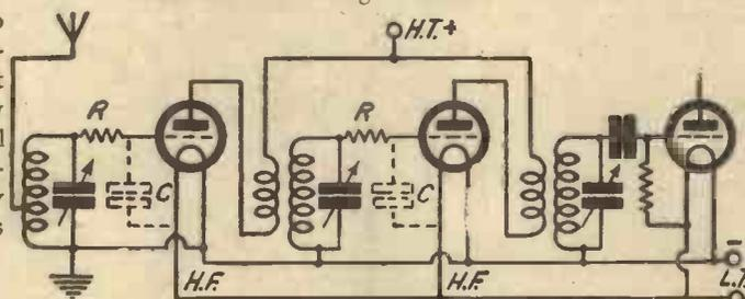
A grid resistance used for stabilising
