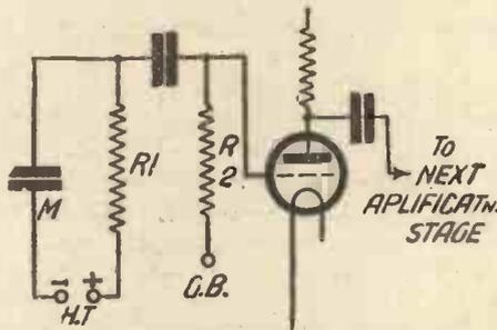
Fig. 1. Method of coupling Condenser Microphone
