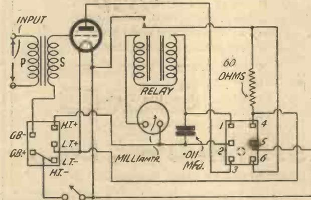
The Circuit Diagram of the Fultograph Relay Panel
