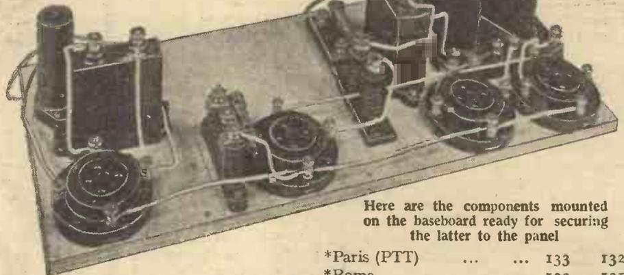
Here are the components mounted on the baseboard ready for securing the latter to the panel
