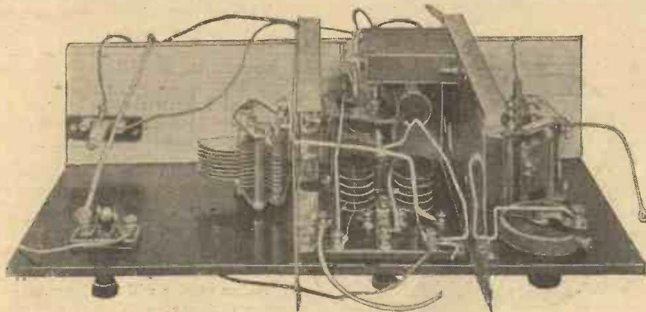
The first stage in the assembly and wiring—the components on the panel
