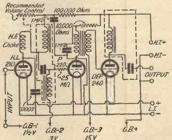
Fig. 2. The Circuit of the Amplifier
