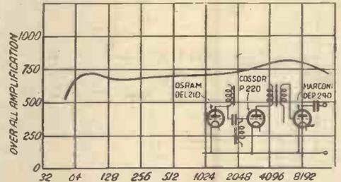
Fig. 1. The Response Curve of the Amplifier
