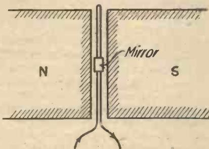
Fig. 1. Principle of the Duddell oscillograph
