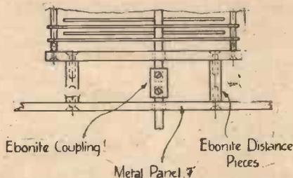
Fig. 1. Condenser mounted on ebonite stand-off insulators
