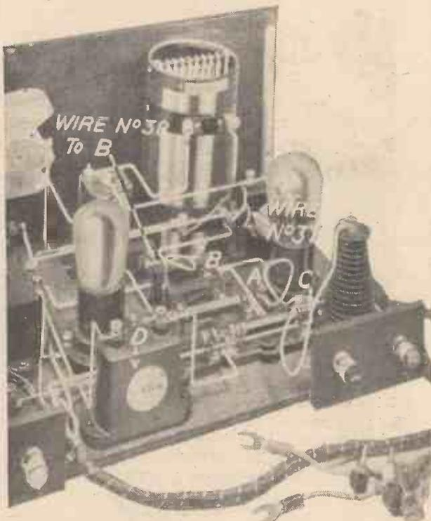
To change over from the long-distance to the local set, remove the four flex leads, leave two free and connect the others to the points indicated
