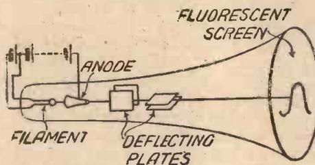
Fig. 1. Cathode-ray Oscillograph
