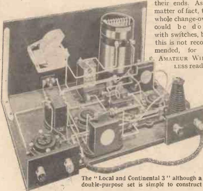
The "Local and Continental 3" although a double-purpose set is simple to construct
