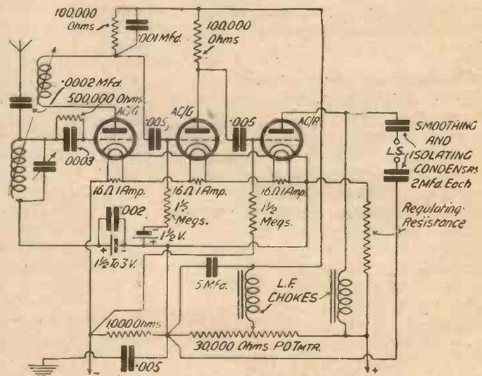
Fig. 4. A 3-valve circuit using indirectly-heated valves
