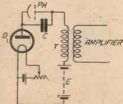
Fig. 2. Photo-cell with two-electrode Valve
