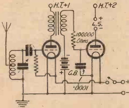
Fig. 1. Where to insert an H.F. stopping resistance
