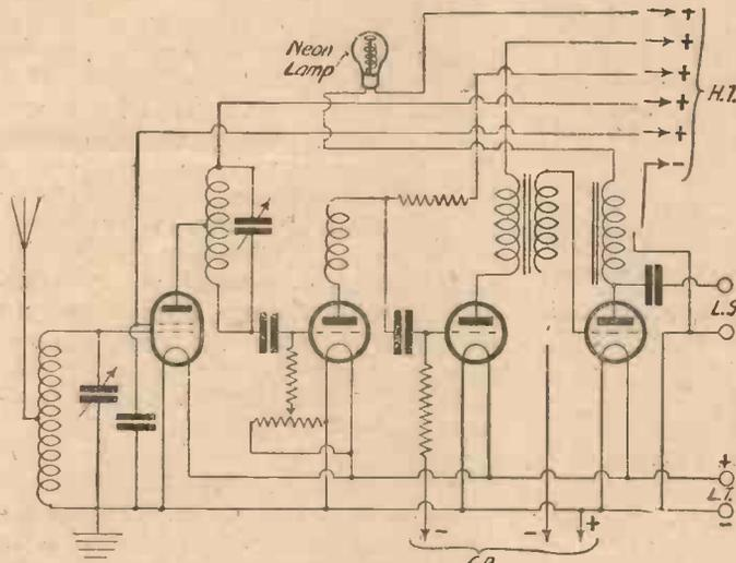
Four-valve circuit showing where the Neon lamp is inserted
