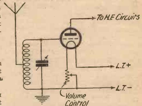
Fig. 2.—Method of controlling H.F.
