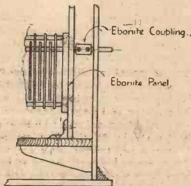
Fig. 2. Condenser mounted on small secondary ebonite panel
