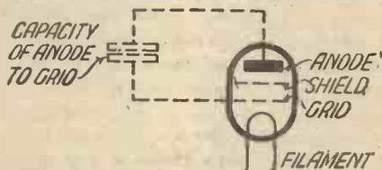
Where there are inter-electrode capacities in a screen-grid valve
