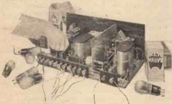
It may be necessary to install in the last holder a valve of lower impedance
