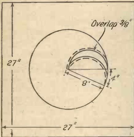
Diagram showing method of cutting diaphragm
