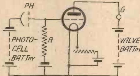
Fig. 1. A Basic Photo-cell Circuit
