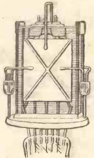
Finally, observe the construction of the anode. Two rectangular nickel plates are used ribbed for greater rigidity.
