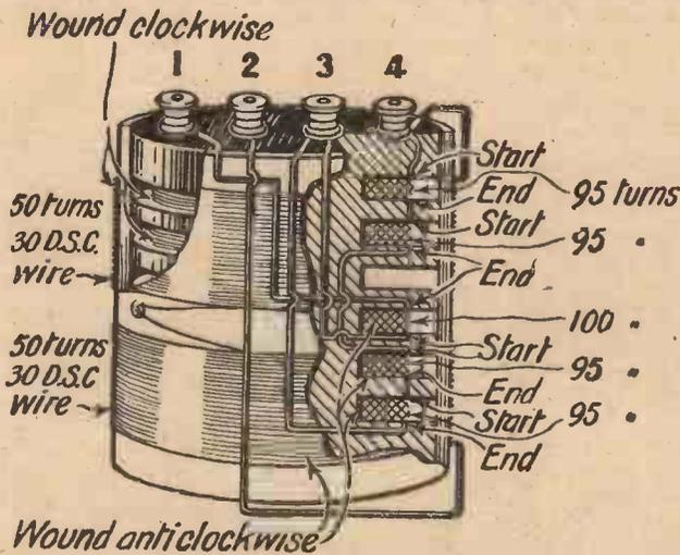
This diagram shows all the necessary constructional details
