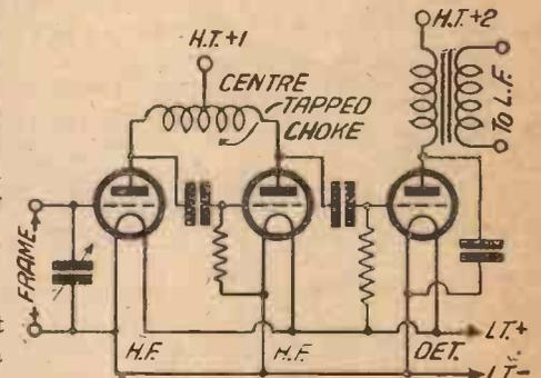
Fig. 2. Simple way of saving an H.F. choke
