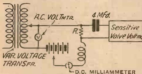
Circuit for Measuring Choke Inductance
