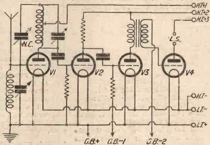
Fig. 2. Typical 4-valve circuit
