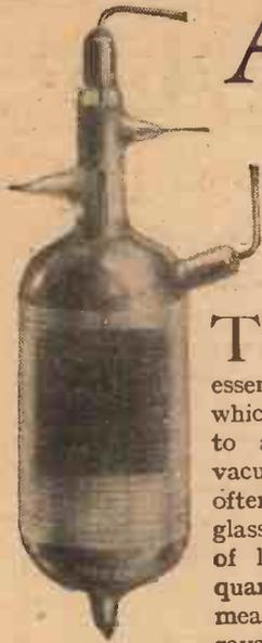
THE photo-electric cell proper consists essentially of a bulb which is evacuated to an almost perfect vacuum. The bulb is often made of pyrex glass, and sometimes of lime glass, and of quartz where it is to measure ultra-violet rays. The lead wires
