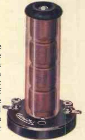
The self capacity of this choke is extremely low owing to the sectional cross windings given on our own special machines. It will improve the range, the volume and the stability of the majority of receivers. **5/-** EACH
