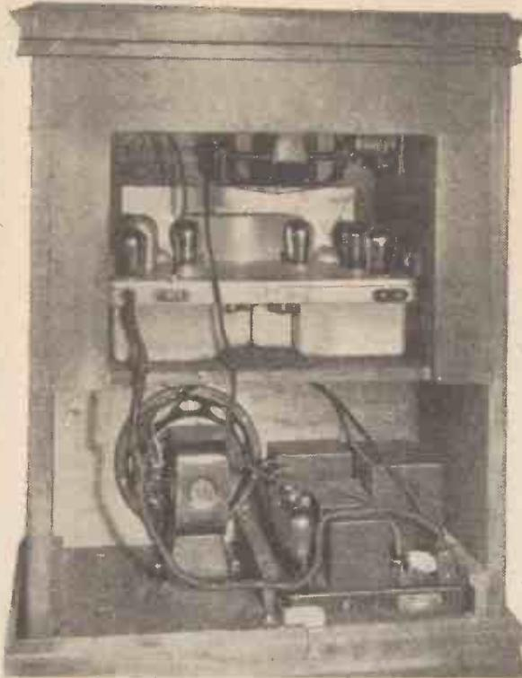
A rear view of a typical American receiver—the Victor. Note the efficient screening
