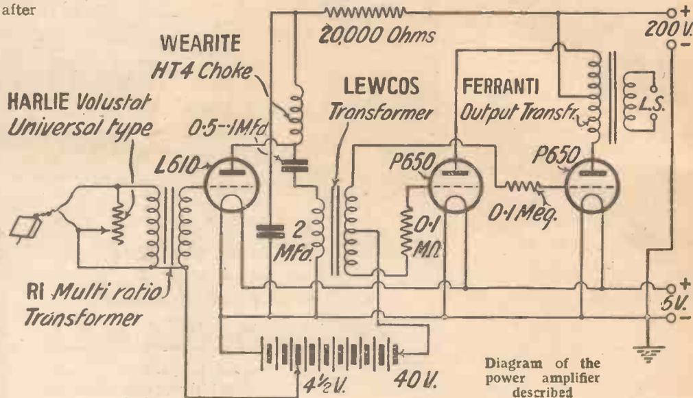
in the neighbourhood of 15 and an A.C. resistance not exceeding 15,000 ohms. It should further be able to handle 4 or 5 volts grid swing and be provided, therefore, with  $4\frac{1}{2}$  volts grid bias. Such a valve as the Osram L610 is suitable in this position.
