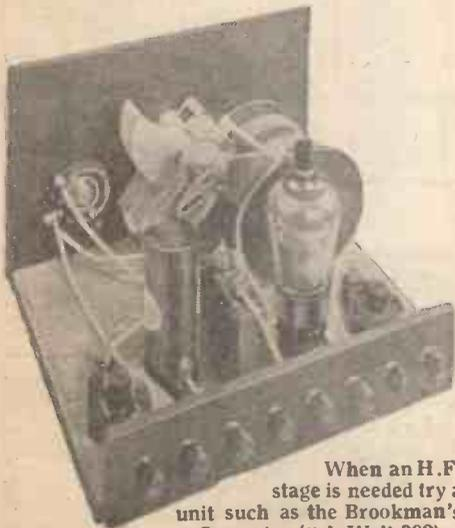
When an H.F. stage is needed try a unit such as the Brookman's Separator (“A.W.” 392)
