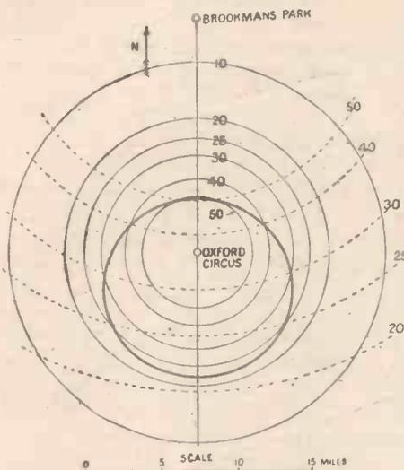
Fig. 3. Circle of equal signals based on field strength
