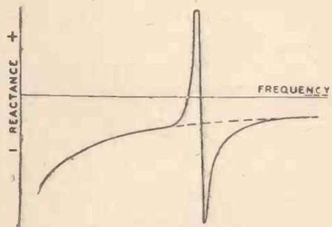
Fig. 3. Reactance curve of oscillator system
