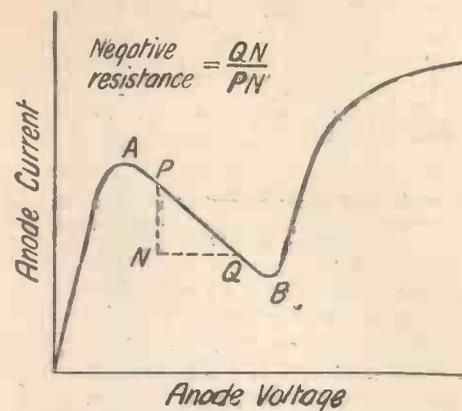
Curve showing anode current and anode voltage for a definite value of grid bias
