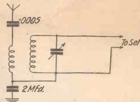
A safety condenser arrangement which should be employed when direct-current mains are used to supply H.T. to a set
