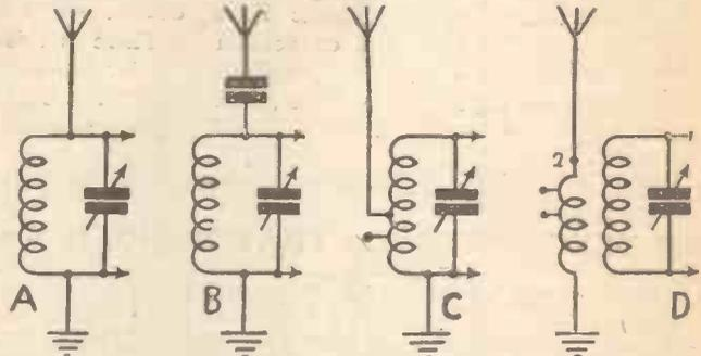
Different types of aerial circuit for obtaining selectivity (A) Usual circuit (B) Series condenser (C) Tapped coil (D) Tapped coupled circuit
