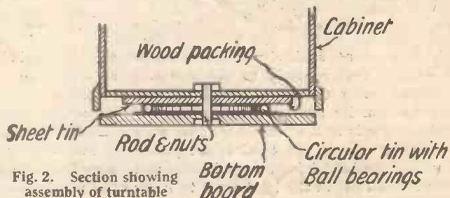
Fig. 2. Section showing assembly of turntable
