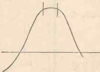
Fig. 2. The armature can rotate an appreciable distance with little variation of the current
