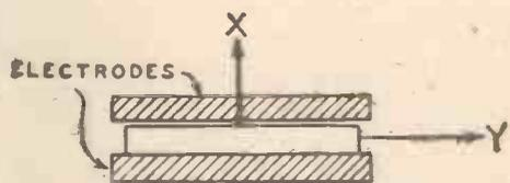
Fig. 1b. Positions of electrodes
