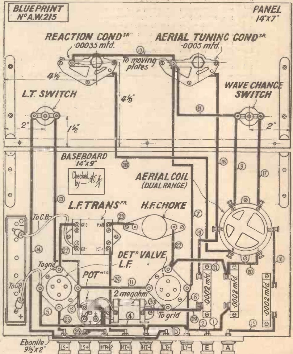
The wiring diagram of the “British Broadcast 2.” A blueprint is available, price 1/-
