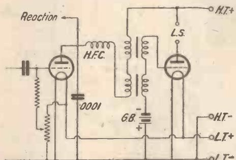
Fig. 2. Getting the effect of a large-ratio transformer by the use of two standard instruments
