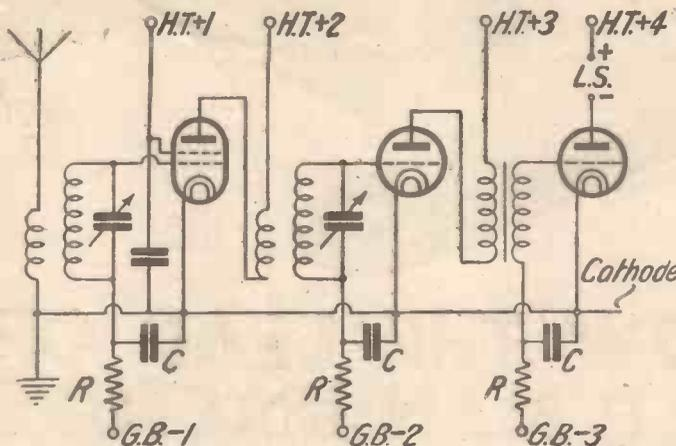
A useful arrangement to prevent mains hum when G.B. is obtained from the power supply
