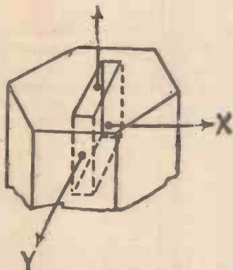
Fig. 1a. Method of cutting crystal
