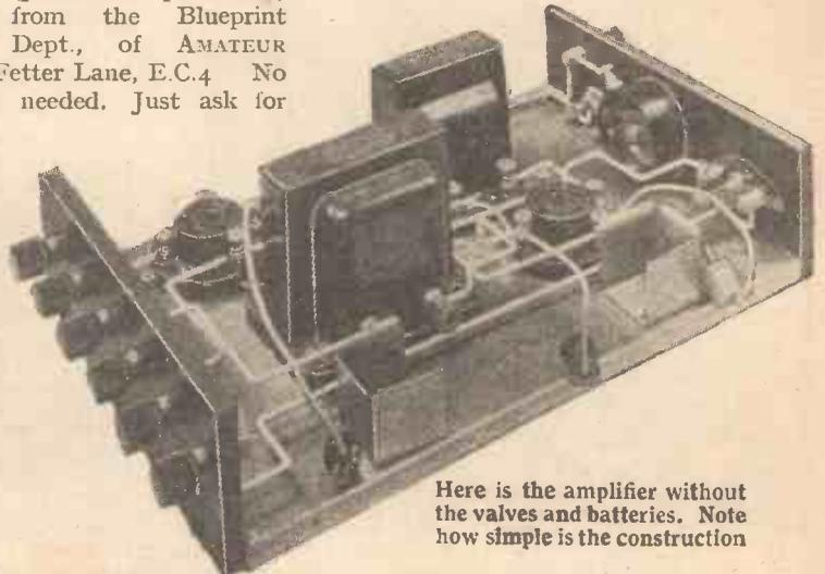
Here is the amplifier without the valves and batteries. Note how simple is the construction
