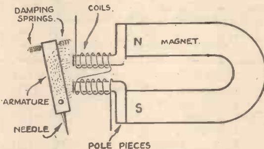
Schematic diagram of moving-iron armature pick-up. Note the change in the number of lines of force when the armature is moved
