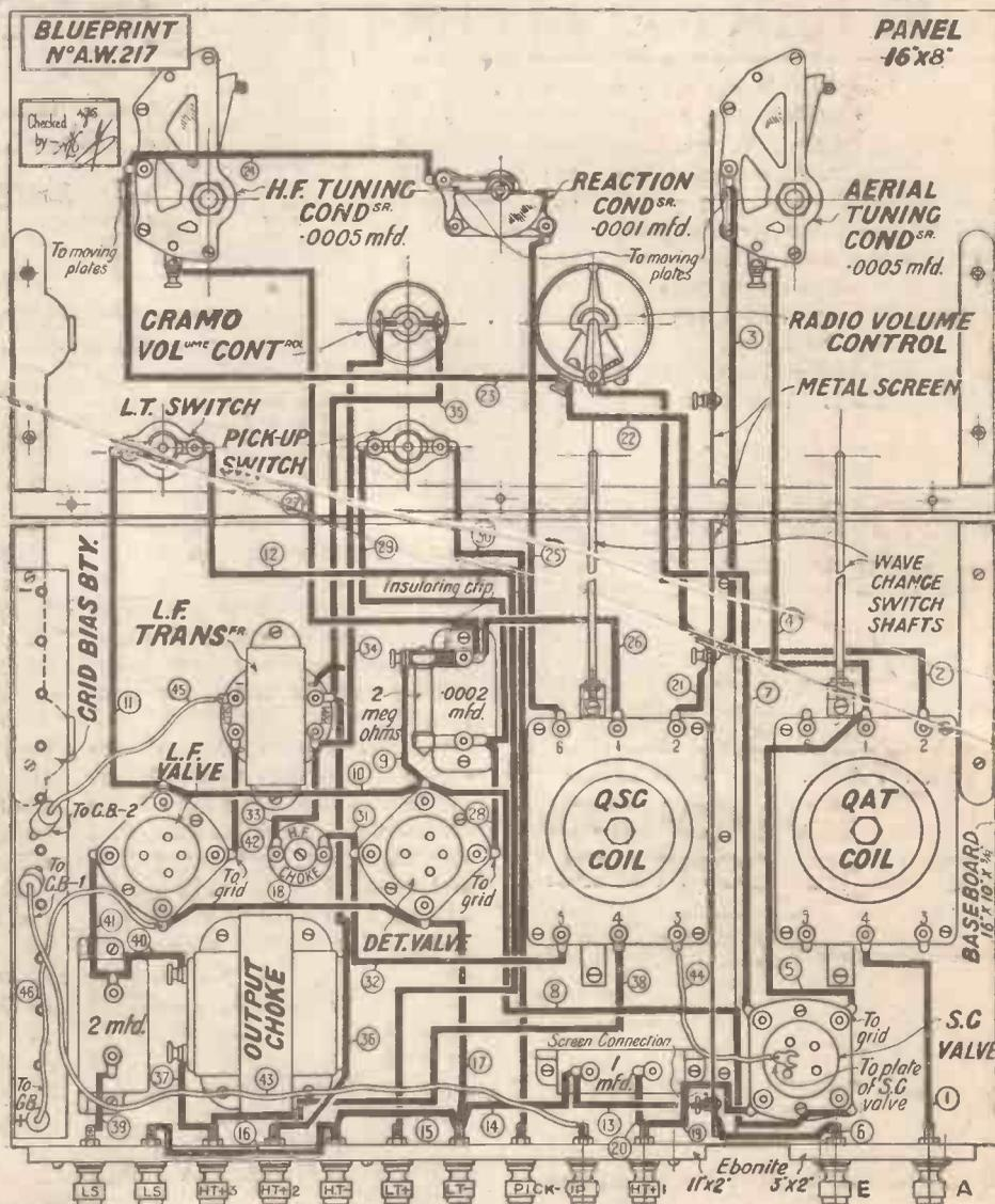
The wiring diagram of which a full-size Blueprint is presented free with every copy of this issue
