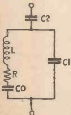
Fig. 2. Electrical circuit equivalent to Quartz oscillator
