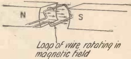
Fig. 1. Principle of the alternator
