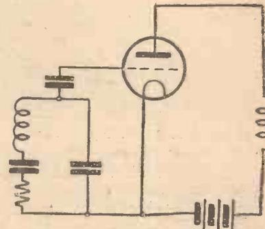
Fig. 4b. The equivalent electrical circuit of Fig. 4a
