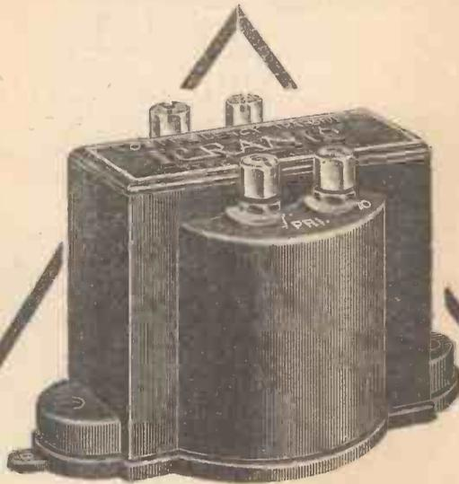
Obtainable in two ratios 3-1 and 6-1. Ratio 3-1 for valves with impedances of 10,000-20,000 ohms. Ratio 6-1 for valves with impedances of 5,000-10,000 ohms.
