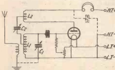
Fig. 1. A simple single-valve constant-coupled circuit
