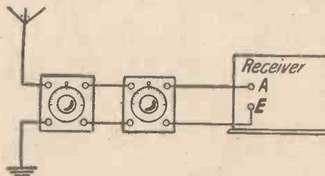
Diagram showing how two by-pass units may be used at the same time
