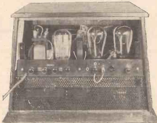
The accessibility of the receiving valves and valve rectifier is clearly shown in this view of the back of the Varley All-electric Two-valve set.
