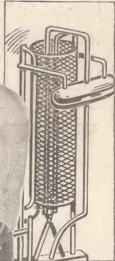
**NOTE** the gauze anode which assists in the ready dissipation of heat and maintains the initial efficiency of the valve throughout a long and useful life.
