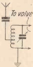
Fig. 4. An ordinary aerial circuit having a tapped coil and series condenser
