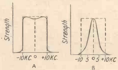
Fig. 3. (A) Tuning curves of properly adjusted coupled circuit. (B) Curve of a single circuit
