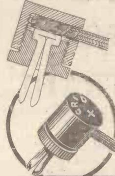
The Powerful grip of the Belling-Lee Wanders Plug and its adaptability to any size battery socket are due to the long prongs made of special spring metal.
