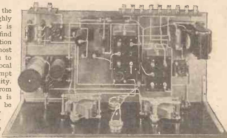
A plan view showing the general layout. The two tapped chokes are clearly shown
