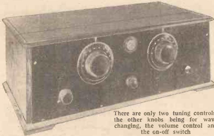
There are only two tuning controls, the other knobs being for wave changing, the volume control and the on-off switch
