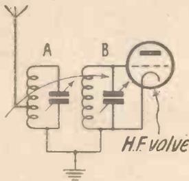
Fig. 2. A coupled aerial-grid circuit
