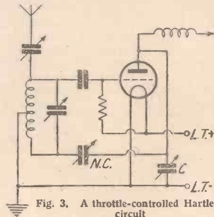
Fig. 3. A throttle-controlled Hartley circuit
