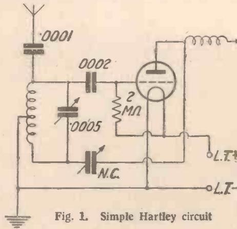
Fig. 1. Simple Hartley circuit
