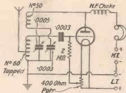
One-valve reaction circuit with potentiometer grid-leak connection
