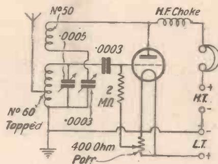
One-valve reaction circuit with potentiometer grid-leak connection
