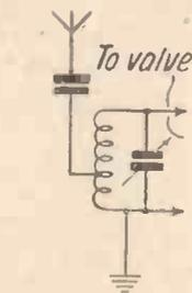
Fig. 4. An ordinary aerial circuit having a tapped coil and series condenser
