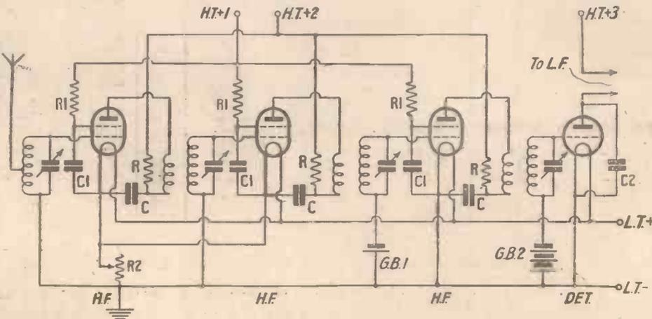
H.F. Amplification is very popular nowadays owing to the need for selectivity. This circuit shows how three H.F. stages can be used, and the various points are explained in the accompanying paragraph
