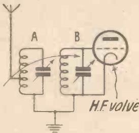
Fig. 2. A coupled aerial-grid circuit
