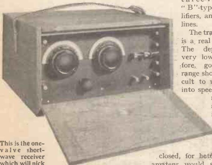
This is the one-valve short-wave receiver which will pick up the transmission from the B.B.C. launch. It is connected through an L.F. amplifier to Savoy Hill
