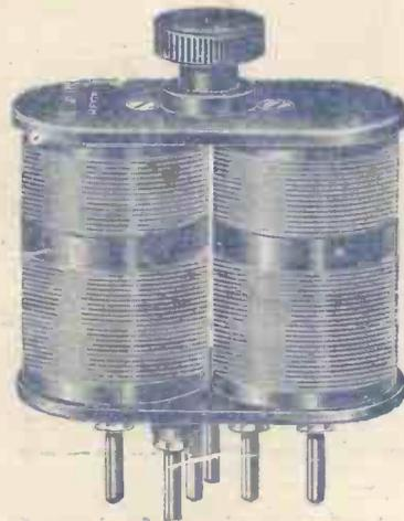
BINOCULAR ABSORPTION WAVE-TRAP
