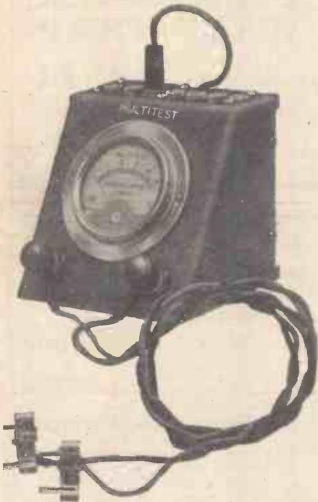
Dead beat Moving Coil. It can be used as a Milliammeter, Ammeter, Voltmeter, Resistance Tester, Cell-testing Voltmeter, Earth-leakage Indicator, etc., etc.
