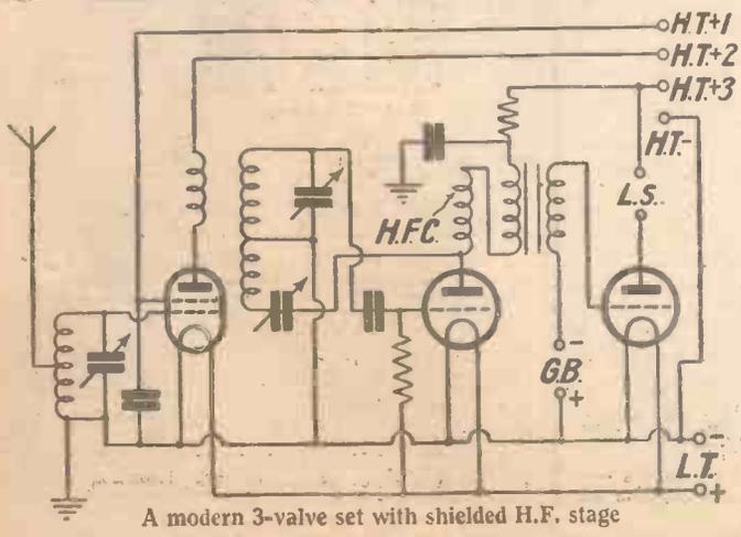
A modern 3-valve set with shielded H.F. stage
