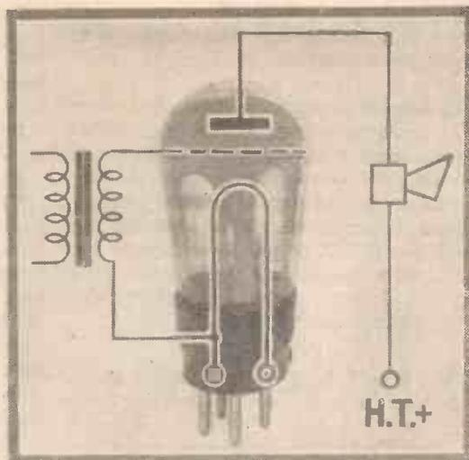
Here is the arrangement when an L.F. valve is used
