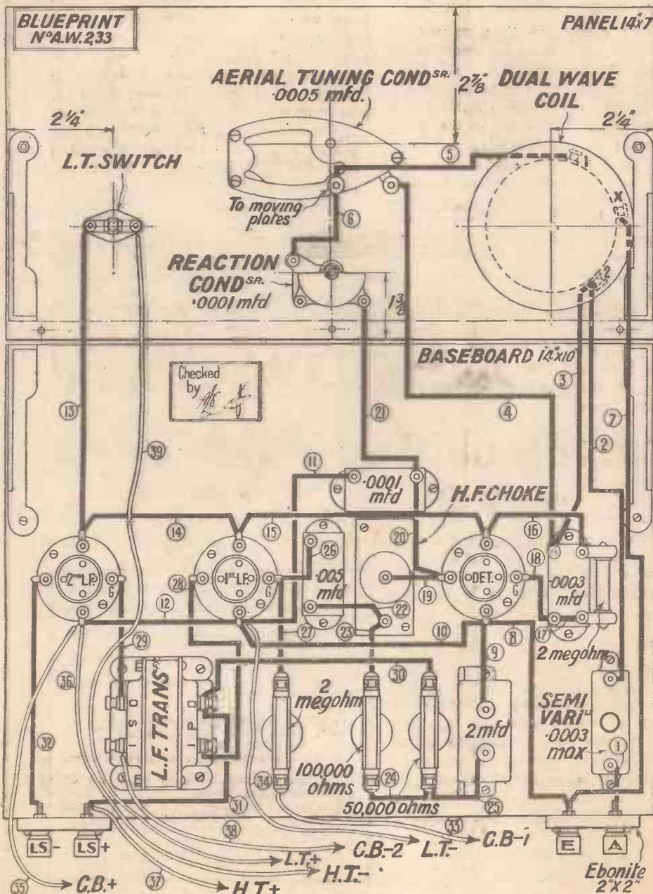
The wiring diagram of the “Beginner’s Regional 3.” A full-size blueprint, which can be had for 1/6, will facilitate construction
