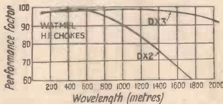
The characteristics of the Watmel chokes tested
