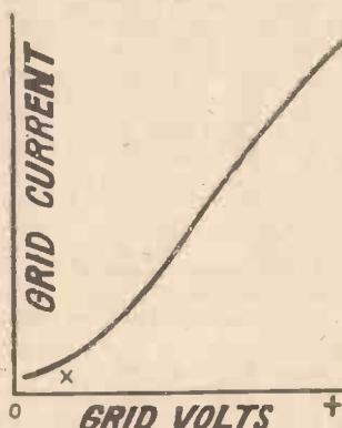
Fig. 3. Note how the grid current increases as the grid voltage is increased
