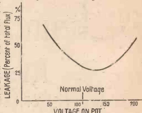
Fig. 2. Curve showing field strengths at different voltages
