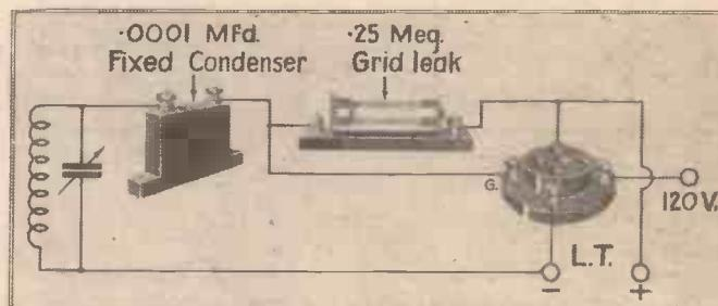
Fig. 2. For power-grid detection low values of grid leak and condenser must be used
