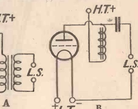
the grid; negative, that is to say, with respect to the negative end of the filament. Low-frequency valves have to be so biased to handle without distortion the large signal voltages developed by preceding valves.
