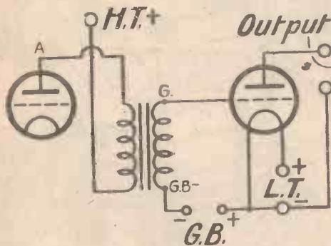
Fig. 2. Two valves coupled by transformer
