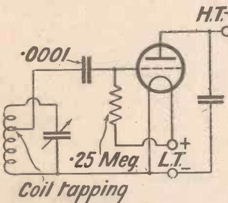
Fig. 4. The tapped coil shown here overcomes the loss incurred by grid-leak damping
