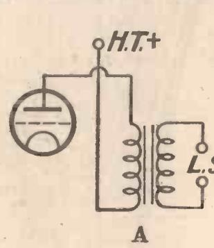
Fig. 4. How a de-coupling arrangement is incorporated
