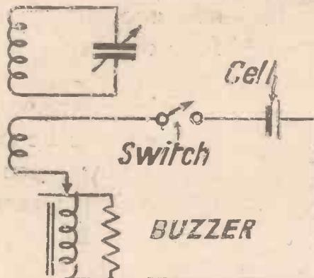
This is the circuit of the handy wavemeter referred to in the accompanying paragraph above. We have first the tuned circuit proper, comprising the coil and adjustable condenser. This circuit may have any type of plain coil and the condenser may be of .0005 microfarads.
