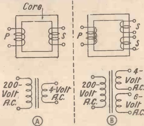
Fig. 1. Simple transformer connections
