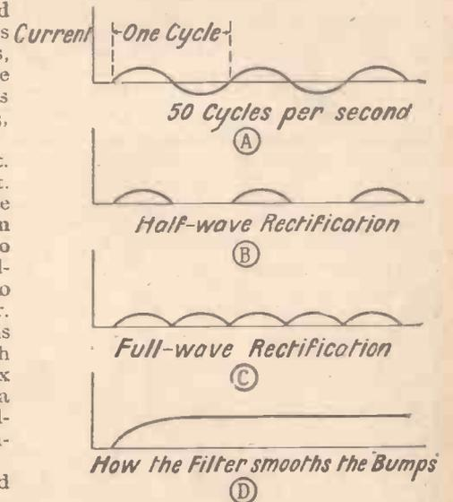
Fig. 3. How the A.C. is converted into D.C.
