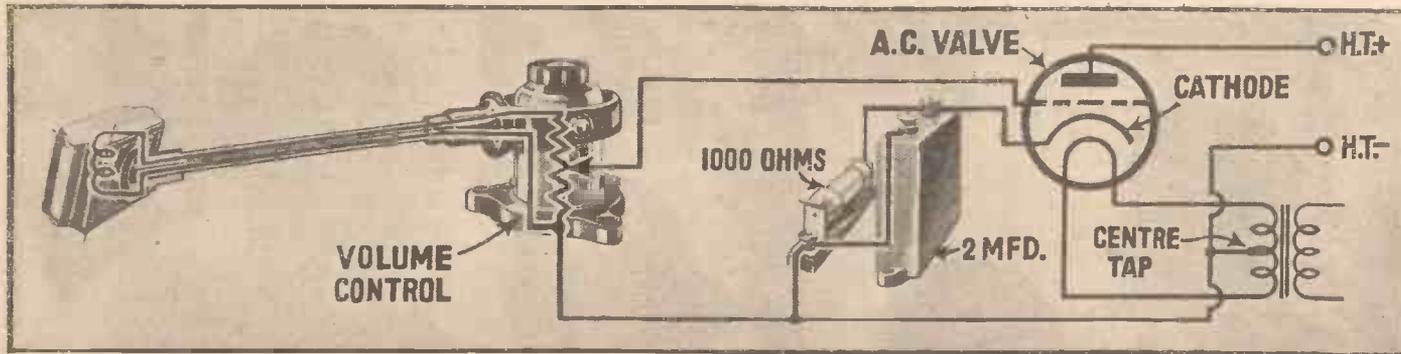
This pictorial diagram shows how "automatic" grid bias can be applied to the first A.C. valve in a gramophone amplifier. Note the volume control between this valve and the pick-up
