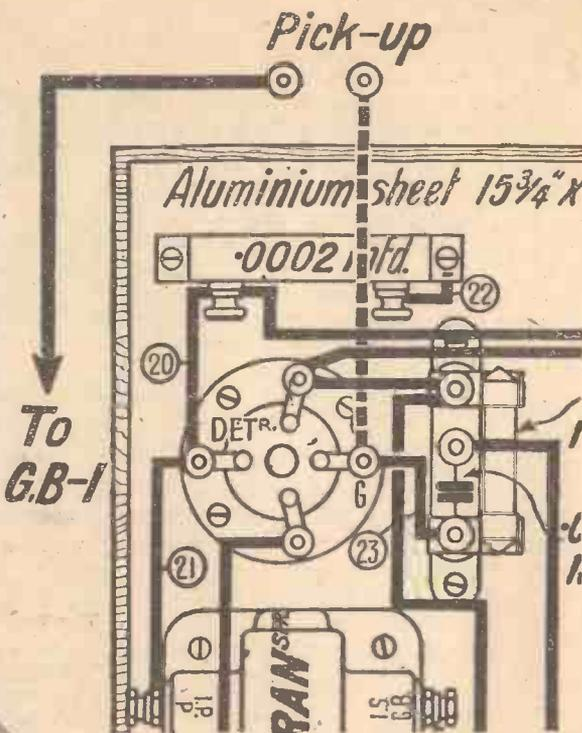
This is a reproduction of a portion of the wiring plan, showing how easy it is to add a pick-up
