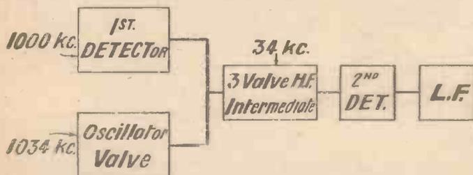
Showing how an incoming signal of 1,000 kilocycles (300 metres) is combined with a local oscillation of 1,034 kilocycles to produce a modulated beat frequency of 34 kilocycles (8,000 metres). This is passed through the long-wave amplifier to the second detector and then amplified in the usual way
