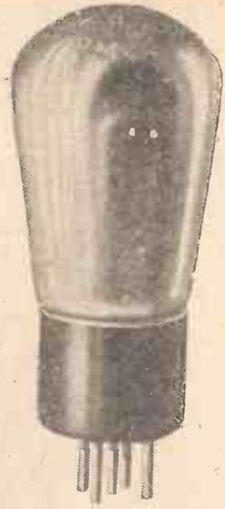
The pentode valve actually provides the output of a super-power valve of the three-electrode class with less input. It must, however, be worked under suitable conditions which are detailed in this helpful article.
