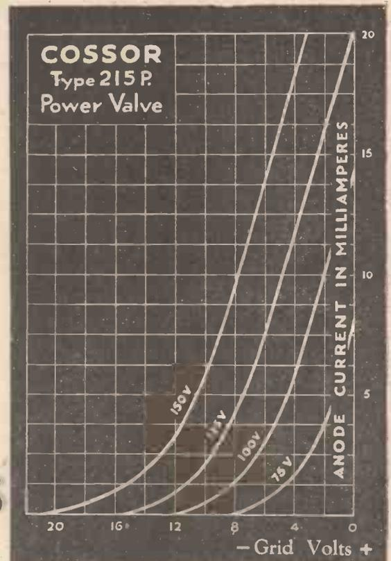
THE quality of the reproduction of your Receiver is largely controlled by its output valve which is called upon to handle very considerable grid swings. If it is unable to do this, distortion is inevitable.
