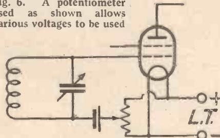
in the case of the Mazda and Eta valves to a small negative voltage in the case of the Cossor valve. In the case of the Mazda and Eta valves one could reasonably use this without any grid bias, provided the input was small. With the Mullard and Marconi valves, grid current begins to lift at zero grid volts, therefore it would appear desir-
