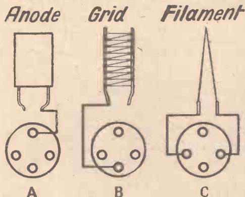
Fig. 2. Connections for anode, grid and filament of three-electrode valves
