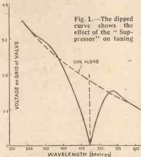
Fig. 1.—The dipped curve shows the effect of the "Suppressor" on tuning
