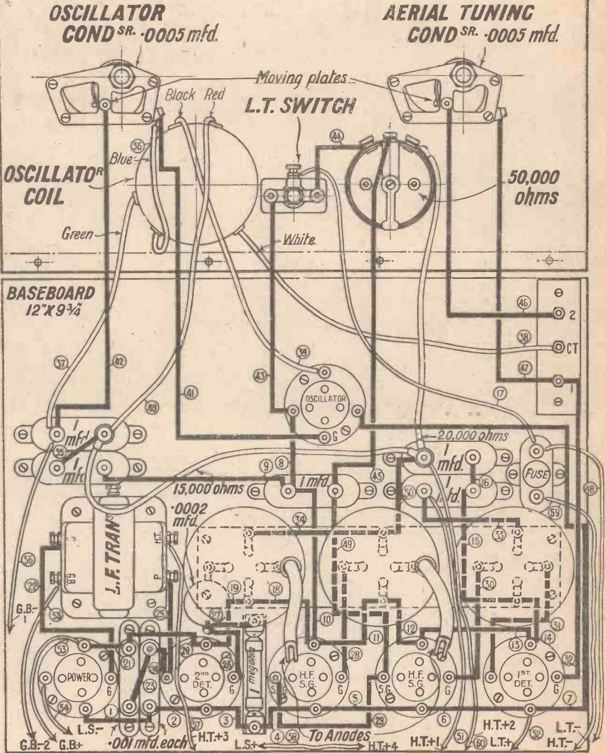
The layout and wiring diagram.
