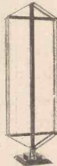
The Lewcos frame aerial which incorporates a neat switching arrangement for medium and long waves
