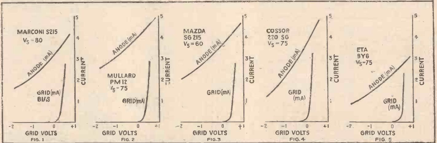
Figs. 1 to 5. Characteristic curves of some typical screen-grid valves
