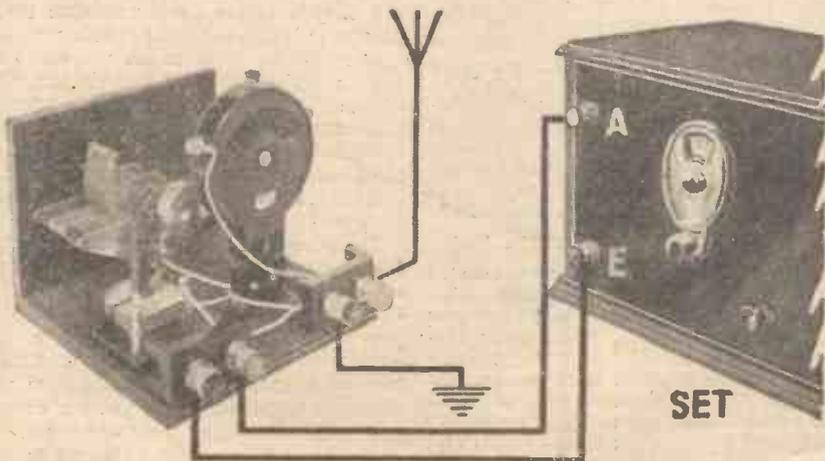
This pictorial diagram shows how the unit is connected to the aerial, earth and the set
