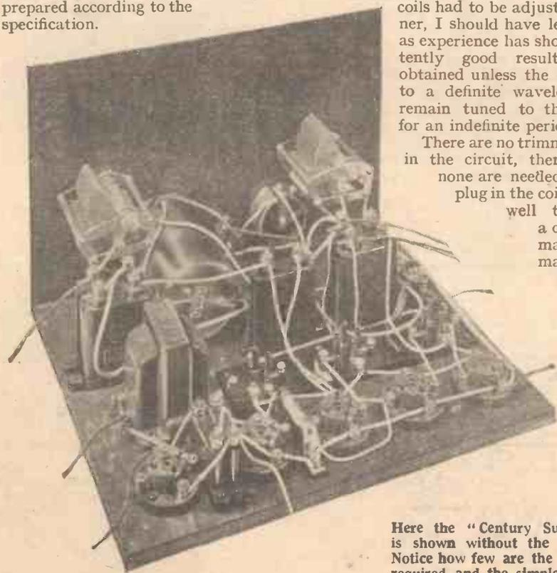
Here the "Century Super" is shown without the coils. Notice how few are the parts required, and the simple construction
