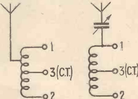
Fig. 1. Balancing condenser in aerial lead
