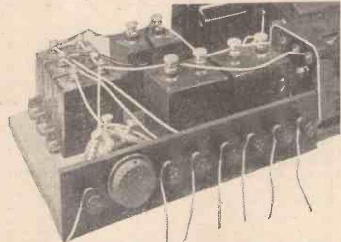
Don't use a mains unit with too few high-tension tapings. This H.T. unit for the "Ether Searcher" has four separate tapings, and this is a great advantage
