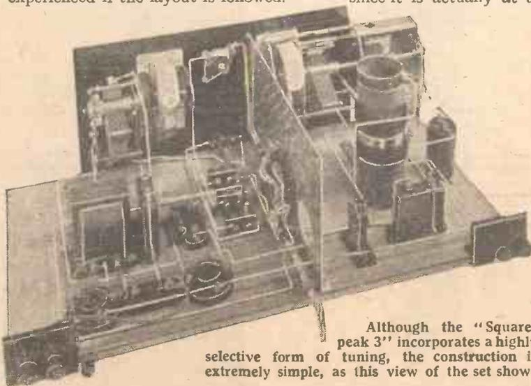
Although the "Square-peak 3" incorporates a highly selective form of tuning, the construction is extremely simple, as this view of the set shows
