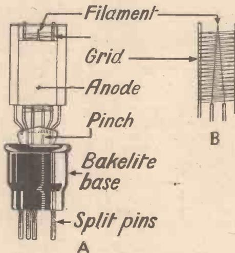
Fig. 1. The construction of a three-electrode valve
