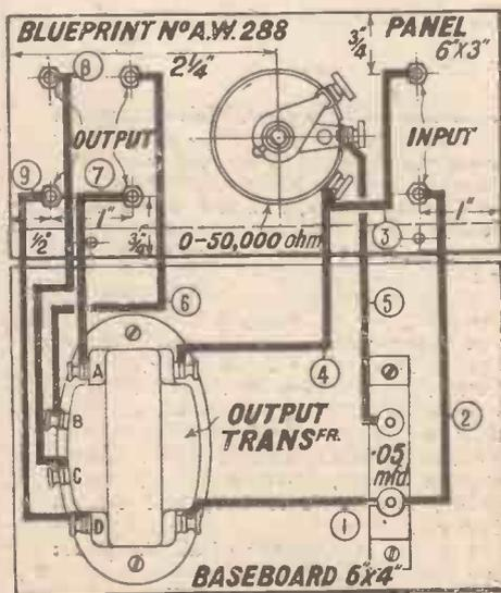
The layout and wiring diagram of the tone changer: A full-size blueprint is available, price 6d.
