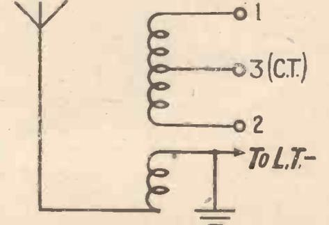
Fig. 2. Coil unit with separate aerial winding
