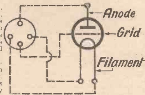
Fig. 3. Comparison between circuit symbol and valve holder
