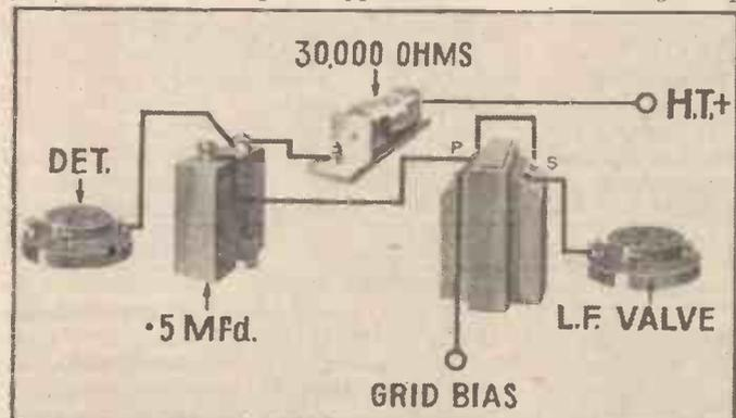
Fig. 1. A suggested alteration—resistance feed for the transformer
