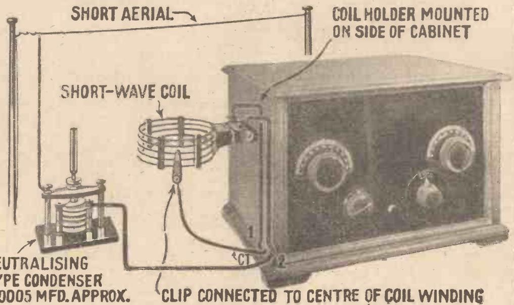
The actual arrangement for short-wave working is shown in this picture. Note the slight modification that is required
