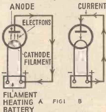
Fig. 1 A and B. Two diagrams showing the part the filament plays in the action of a valve
