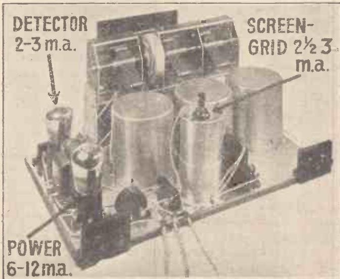
This view of a typical three-valver shows the average current taken by the screen-grid, detector and power valves. The H.T. unit must give sufficient current
