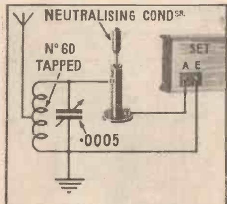
Fig. 2. Adding an external tuned circuit will improve selectivity
