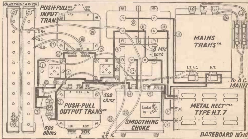
The layout and wiring diagram of the A.C. Push-pull Amplifier. A full-size blueprint is available, price 1/-
