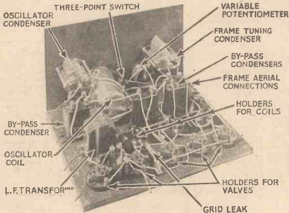
This photograph shows the positions of the various components of the "Century Super" which can be identified in the accompanying list
