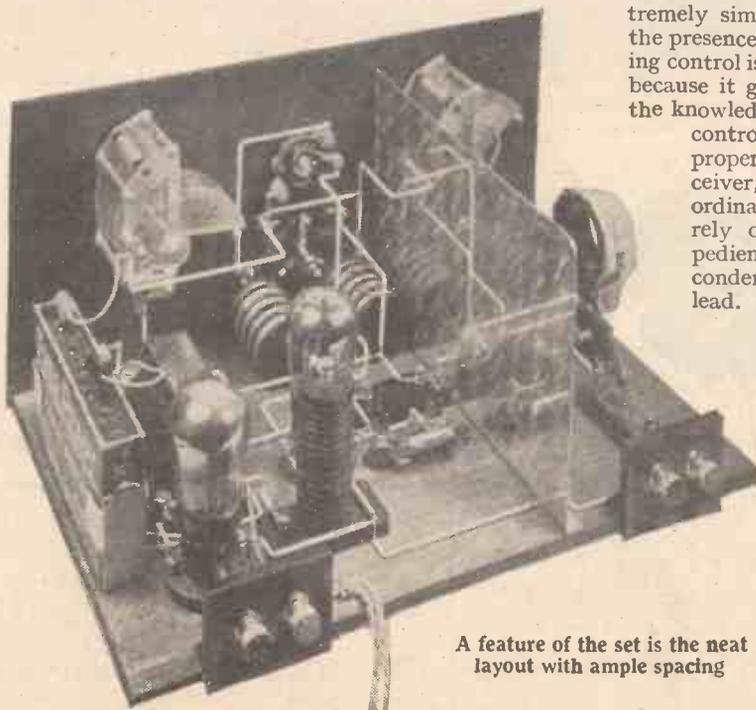
A feature of the set is the neat layout with ample spacing
