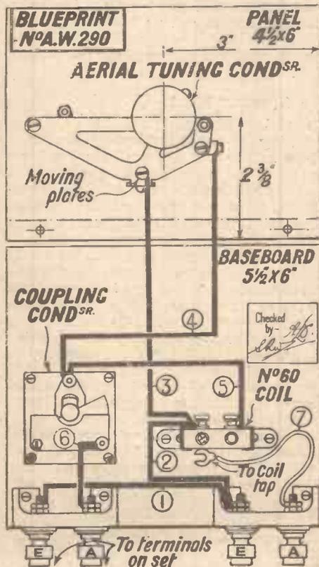
The layout and wiring diagram. A full-size blueprint is available, price 6d.
