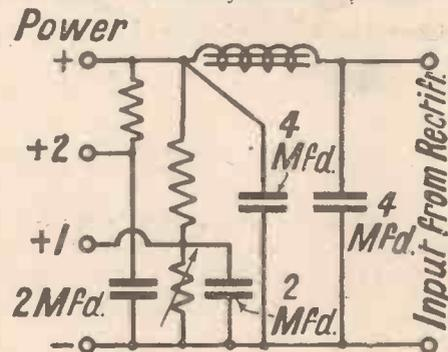
Fig. 2. Circuit arrangements of a suitable mains unit
