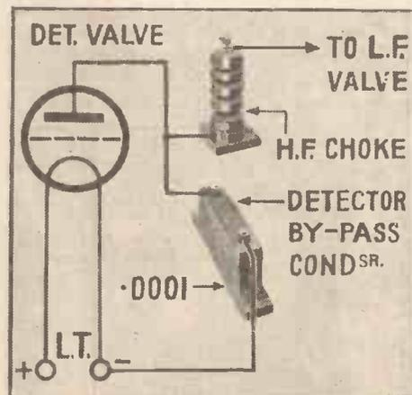
Fig. 3. An anode by-pass condenser will prevent instability
