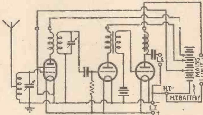
As explained in the accompanying paragraph, it is possible to have a mains unit working in conjunction with a high-tension battery
