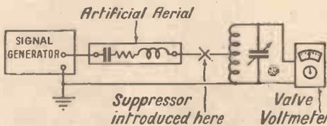
Fig. 2.—Circuit used for testing the "Regional Suppressor"
