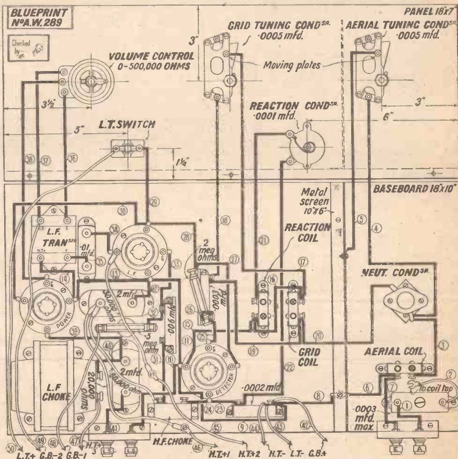
The layout and wiring diagram of the "B.B.C. Selective Three." A full-size blueprint is available, price 1/-
