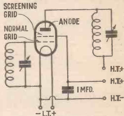
Fig. 2. Connections of screen-grid valve in tuned-anode circuit
