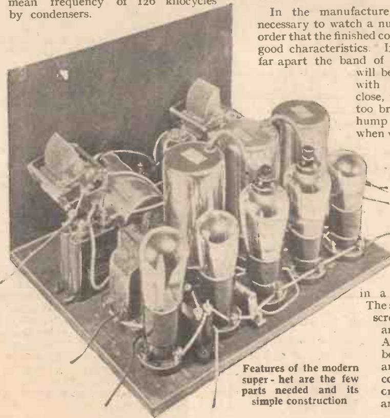
Features of the modern super-het are the few parts needed and its simple construction
