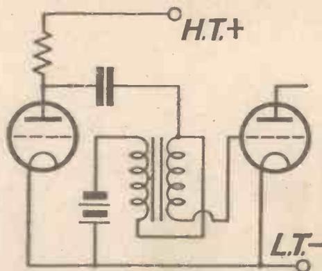
This is the special resistance-feed circuit for an L.F. transformer, referred to by W. James in the accompanying paragraph
