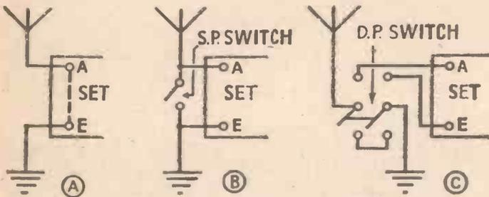
Fig. 1. Three diagrams of aerial arrangements showing how the set can be protected
