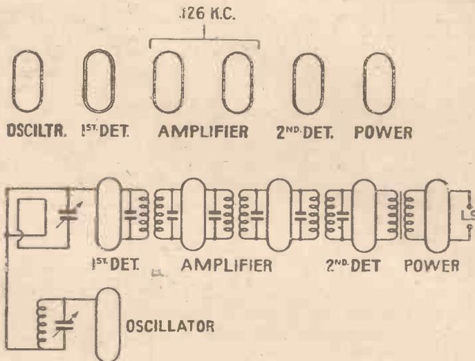
Fig. 1. Arrangement of valves in super-het receiver
