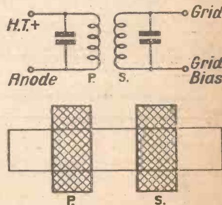
Fig. 2. Band-filter coil for super-het
