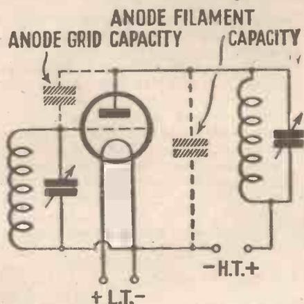
Fig. 1. Connections of three-electrode valve as H.F. amplifier
