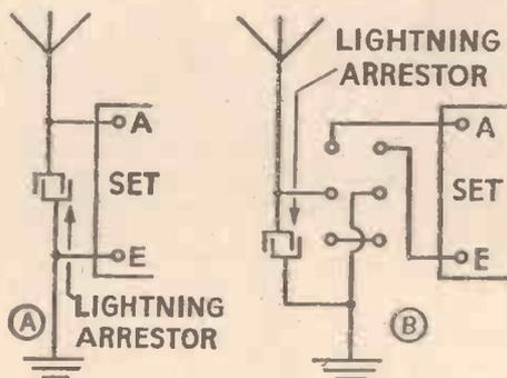
Fig. 2a. How a lightning arrestor is installed. Fig. 2b. Arrangement of lightning arrestor and earthing switch
