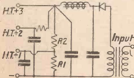
Fig. 3. Circuit showing terminal connections
