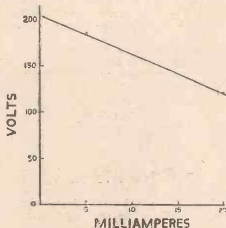
Fig. 2. Output curve of typical mains unit
