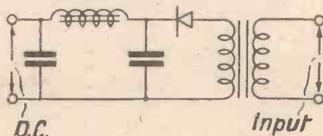
Fig. 1. Circuit of half-wave rectifier
