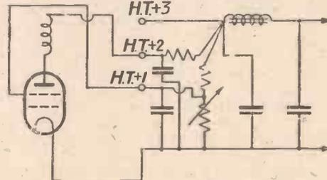
Fig. 4. Connections of mains unit for screen-grid valve
