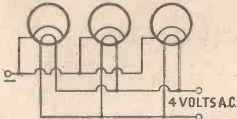
Fig. 1. A.C. Valves working in parallel
