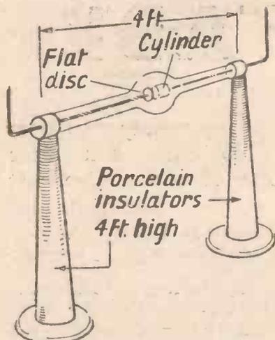
Fig. 1. Diagram of the 100,000-volt rectifier used for X-ray work
