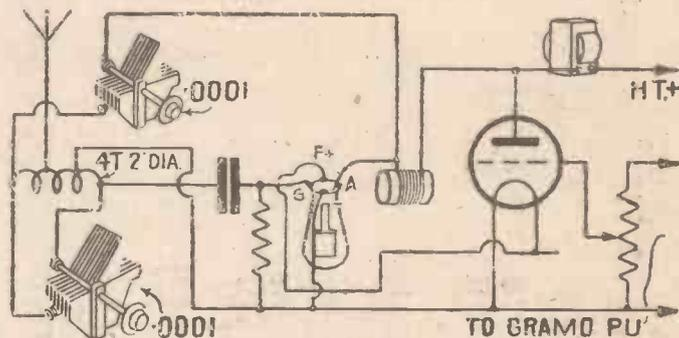
Fig. 2. Schematic diagram of 1 1/2-5-metre transmitter. The receiver is similar except that no modulator valve is required
