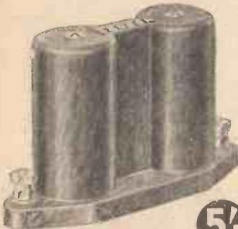
**THE TELSEN BINOCULAR H.F. CHOKE.**—Has an exceptionally high impedance and low capacity resulting in an excellent performance curve. It has a restricted field and covers the whole broadcast. Free from parasitic resonances. Inductance: 180,000 microhenries. Self Capacity: .000002 microfarad. Resistance: 750 ohms. Price 5/- each.
