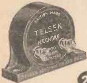
**TELSEN STANDARD H.F. CHOKE.**—Designed to cover the whole broadcast range. Exceptionally low self capacity; inductance 150,000 microhenries; resistance 400 ohms. Price 2/- each.
