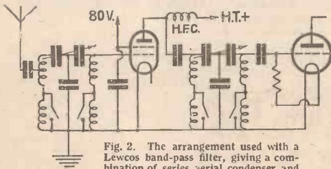
Fig. 2. The arrangement used with a Lewcos band-pass filter, giving a combination of series aerial condenser and a tap on the short waves
