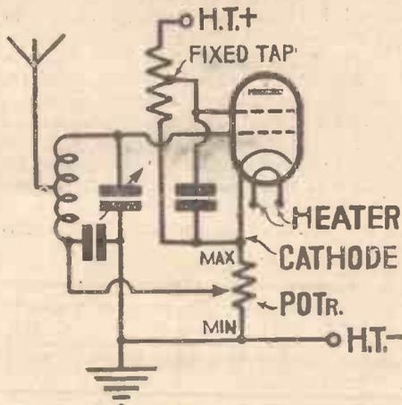
Fig. 7. Connections of volume control for variable-mu valve
