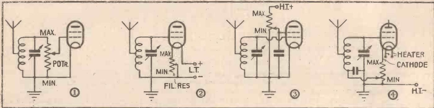
Fig. 1. Input volume control. Fig. 2. Filament resistance volume control. Fig. 3. Screen-grid type volume control. Fig. 4. Grid bias control of A.C. mains screen-grid valve
