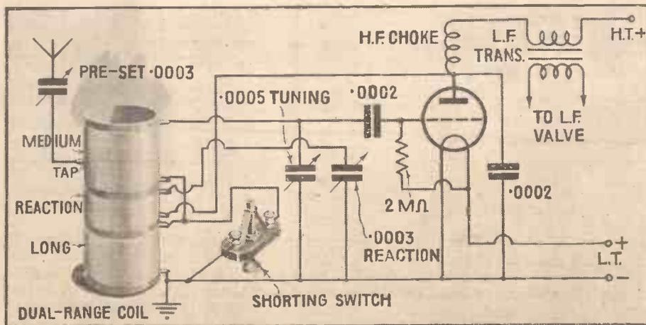
Fig. 4. Suggested circuit for using dual-range coil
