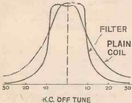
Fig. 1. Resonance curves of plain and band-pass circuits
