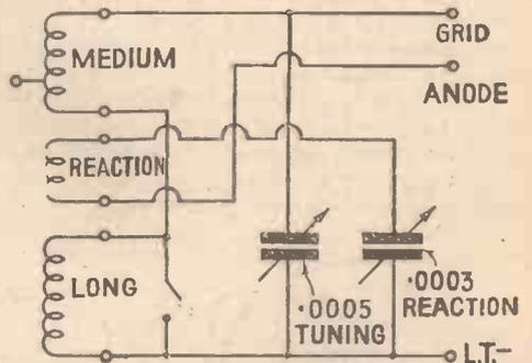
Fig. 2. Dual-range coil with reaction winding
