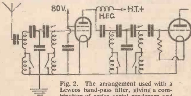
Fig. 2. The arrangement used with a Lewcos band-pass filter, giving a combination of series aerial condenser and a tap on the short waves
