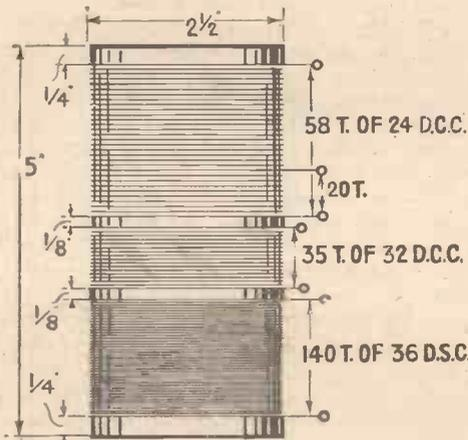
Fig. 3. Winding data for dual-range coil
