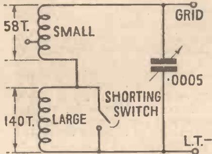
Fig. 1. The connections of a dual-range tuner
