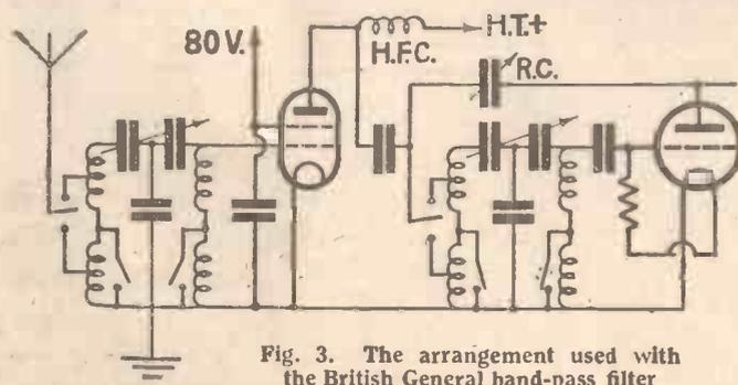
Fig. 3. The arrangement used with the British General band-pass filter
