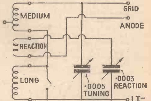
Fig. 2. Dual-range coil with reaction winding
