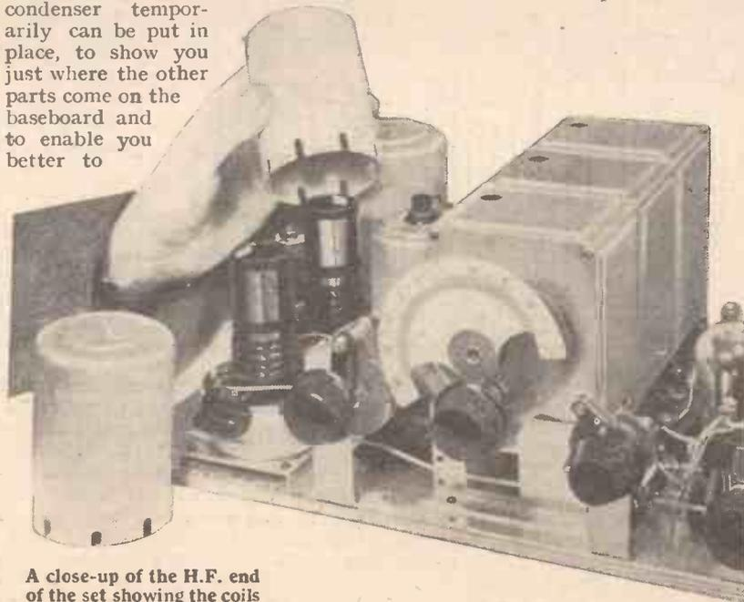
A close-up of the H.F. end of the set showing the coils
