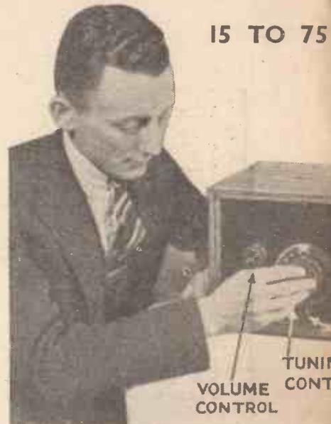
Although a super-het, this set has only one tuning other controls, namely the volume control.
