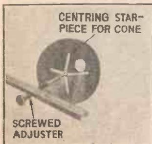
Fig. 4. A simple centring adjustment of particular interest to moving-coil owners
