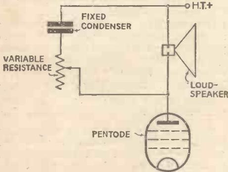
When increasing the amplification of a set by using a pentode instead of an ordinary power valve, remember to add tone-correcting components to avoid high-note accentuation
