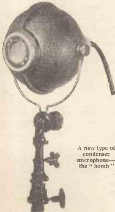
A new type of condenser microphone—the "bomb"
