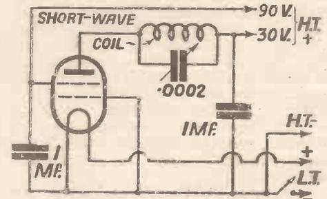
The circuit of the short-wave wavemeter
