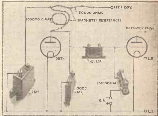
Here is a pictorial diagram showing the skeleton connections for an intermediate stage of resistance-capacity coupling between the detector and power valves. Note the de-coupling condenser and the anode by-pass condenser
