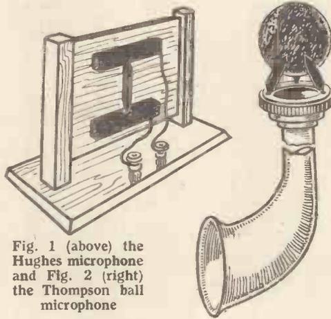
Fig. 1 (above) the Hughes microphone and Fig. 2 (right) the Thompson ball microphone
