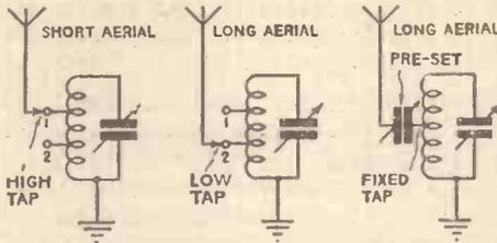
If you lengthen the aerial to improve its efficiency you must take precautions against broad tuning. With a tapped aerial coil a tap nearer to earth will be needed for the aerial lead when using a long wire. If there is no tap on the coil, or this is fixed, you can obtain the same effect by putting in a pre-set condenser
