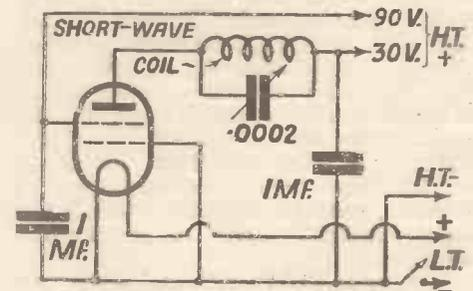
The circuit of the short-wave wavemeter
