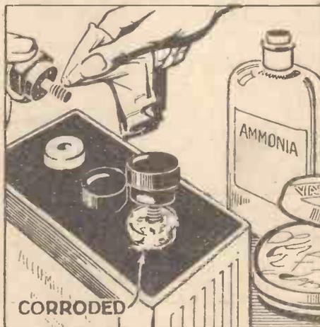
The terminals and top of the battery should be cleaned with ammonia and coated with vaseline
