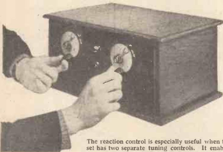
The reaction control is especially useful when the set has two separate tuning controls. It enables the two circuits to be kept "in step" as explained in the accompanying article
