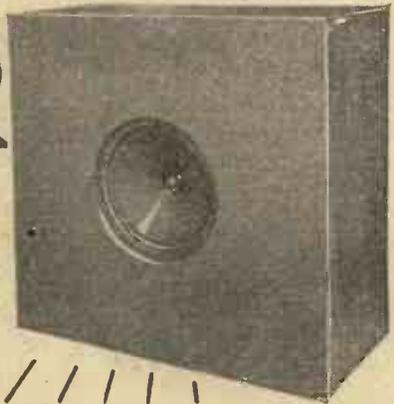
Full constructional details of a new type of baffle first introduced into this country by the B.B.C. to enable natural bass-note reproduction to be obtained with a convenient size of box instead of a large and unwieldy baffle board
