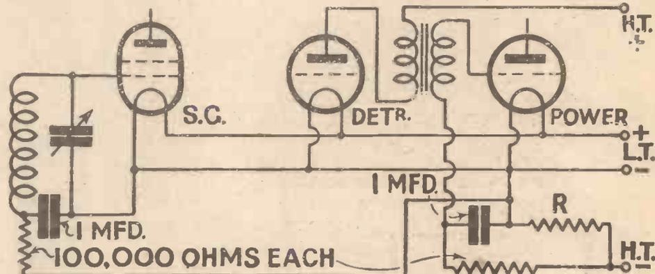
This is a typical three-valve circuit in which automatic bias is applied by means of voltage-dropping resistances
