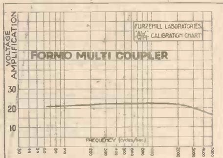
This curve shows the effective amplification of the Formo Multi-coupler plotted against frequency
