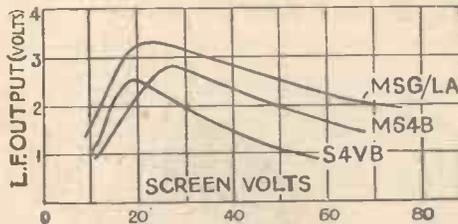
Fig. 5. The optimum screen voltage is more critical with the anode-bend-circuit and is also distinctly lower
