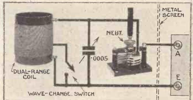
A simple band-pass aerial tuning arrangement can be fitted up with a dual-range coil, a tuning condenser, and a small coupling condenser, as shown by the above pictorial diagram
