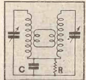
The coupling condenser value c depends upon the type of coil used, but an average value is .05 microfarad. The grid resistance R, the purpose of which is only to complete the grid circuit, can generally be of 1,000 ohms.
