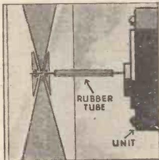
phragms, you sometimes notice a rattle on loud notes. This is due to resonance of the long rod. It is easily cured by slipping a length of valve rubber tubing over the rod.
