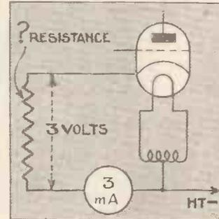
Here is a practical example of the working of Ohm's Law. You want to know the value of resistance for grid bias in a mains valve circuit. It can be found quite easily as you know the voltage required (the grid bias) and the anode current flowing
