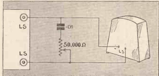
A simple loud-speaker tone control can be made up with a .01-microfarad fixed condenser and a 50,000 ohms variable condenser, connected in series across the speaker terminals
