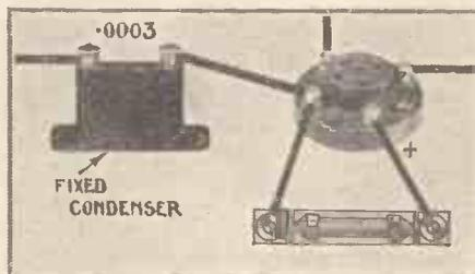
The normal connections for a power valve connected to a low-frequency transformer without a volume control
