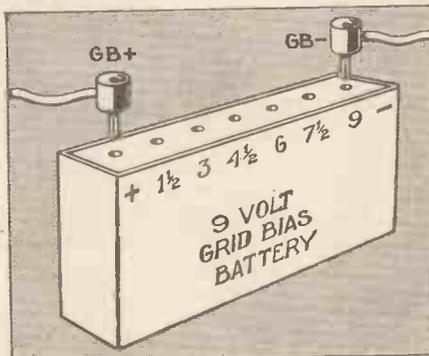
A grid-bias battery, such as that shown above, consists of a number of 1½-volt cells connected in series and provided with tapping points. Into these tapings, which are in the form of sockets, we insert the grid-bias leads connected to plugs. Grid bias is varied by changing the negative socket connections of the plugs
