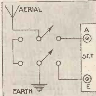
The connections for an efficient aerial-earthing switch are shown above. Fit the switch up outside the house, near the lead-in wire if possible
