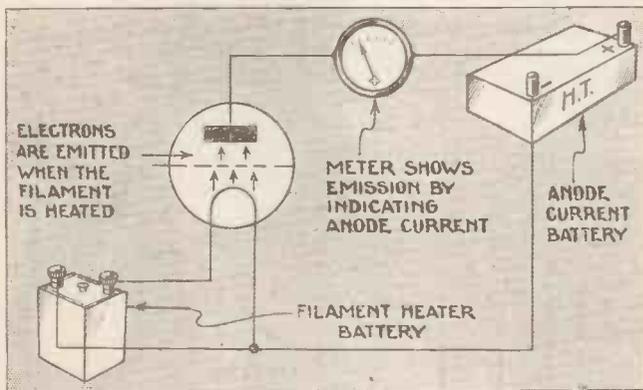
Old valves are expensive to run because, although the filament is heated and therefore draws current from the accumulator, the electron emission from the filament falls off, and so does the overall efficiency of the valve
