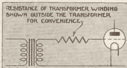
For convenience, the resistance of the low-frequency transformer is shown above as a separate resistance in the grid circuit of the valve following the transformer
