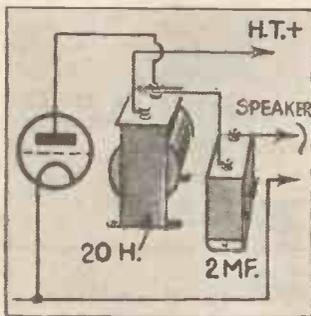
gram. This shows typical values for the average power valve output, and used with a normal speaker. A centre-tapped choke must be used with a pentode, in order to secure proper impedance matching.
