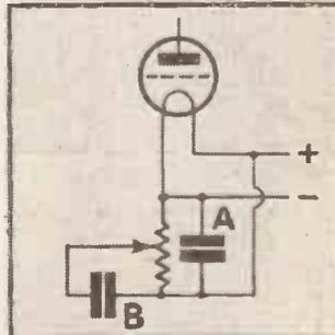
of the bias on the detector grid makes for easy reaction. It is not so well known, however, that a condenser across the "pot" winding is sometimes needed to prevent motor-boating. This condenser is shown at A in the accompanying diagram. An alternative position for the condenser is at B, where it is between the slider and one end of the potentiometer.
