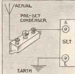
One of the simplest gadgets you can fit to your set is a pre-set type of condenser, as shown in the above diagram. Make sure that the set does not already contain such a device
