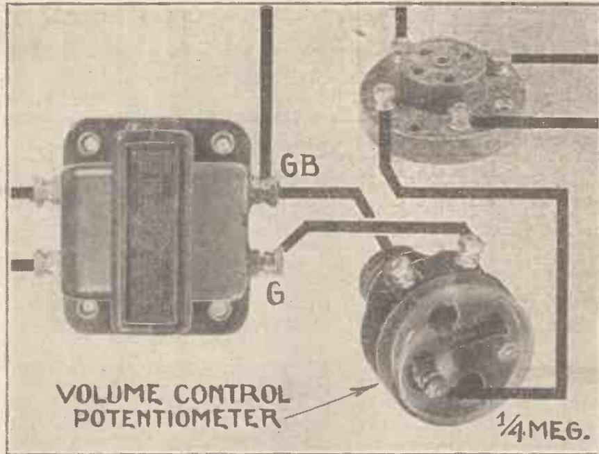
This pictorial diagram shows very clearly how you can fit up a potentiometer between the transformer and the power valve to act as an efficient volume control
