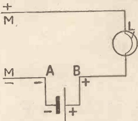
Fig. 1. This shows a lamp being used as a resistance
