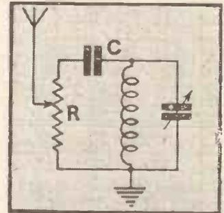
diagram. Various values for the coupling condenser c may be tried; but, generally speaking, a value of .0001 microfarad is satisfactory. A 50,000-ohm potentiometer will do with the slider connected to the aerial. Preferably use a potentiometer which is not too compact and which has not too much metal in its construction. In the diagram the coupling condenser is shown at c and the potentiometer winding at R.
