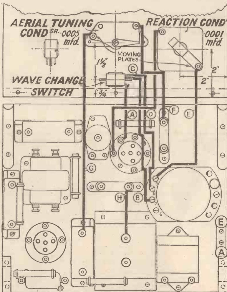
The modified layout and wiring diagram. Wires numbered 1, 2, 4, 5, 6, 37, 38, 39, 40 and 41 shown on the blueprint published last week are omitted and the additional wires, lettered in alphabetical sequence and shown above, added
