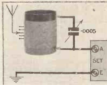
Here is one of the best types of wave-trap, consisting of a tapped coil tuned by a .0005-microfarad variable condenser. Vary the tap and you vary the trapping effect
