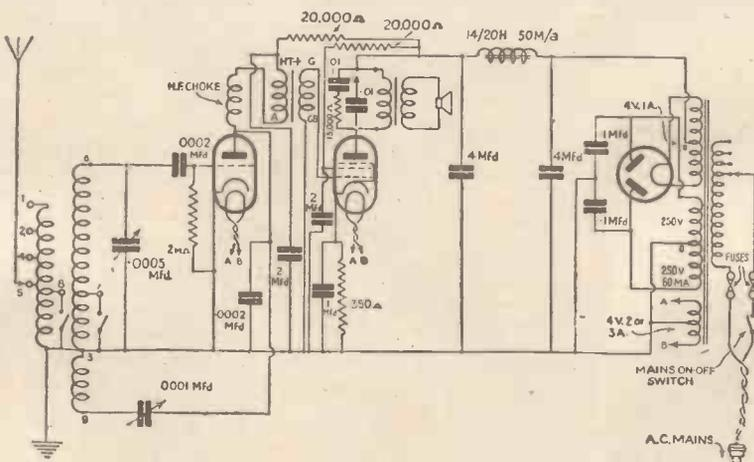
This is the modified circuit which will allow the "Home-station A.C. Two" being tuned on the medium- and long-wave bands
