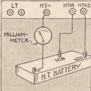
The correct place to connect a milliammeter when you want to find the total anode-current consumption is in the high-tension negative lead. To find what each valve is taking insert the meter in the individual positive leads
