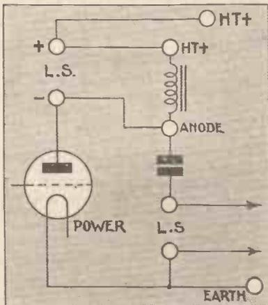
Connections for adding a choke-capacity filter to your set, to isolate the loud-speaker from the direct current of the high-tension battery
