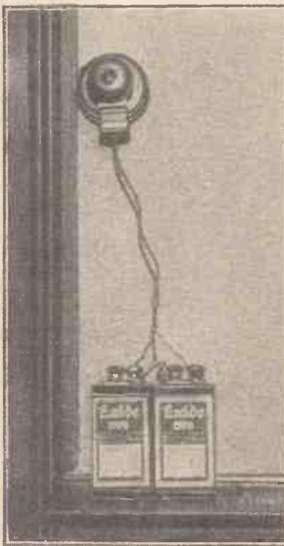
Fig. 3. Here the battery is connected across a switch so that the current used to light the lamp is passed through the accumulator
