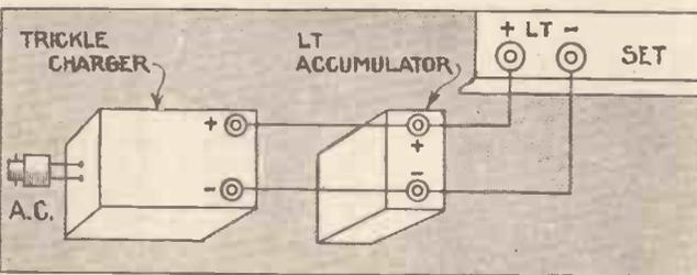
A trickle charger can be permanently connected up to the filament accumulator, but it is essential to switch off the A.C.-mains supply when using the set, otherwise there will be an unbearable background noise due to mains hum
