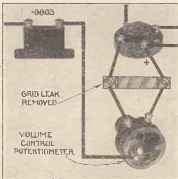
With the aid of a potentiometer volume control you can control the volume by varying the input to the grid of the detector valve, as shown by the above pictorial diagram
