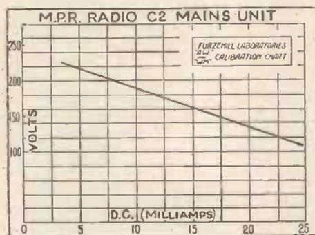
This curve shows the H.T. output obtained from the Mains Power Radio unit tested
