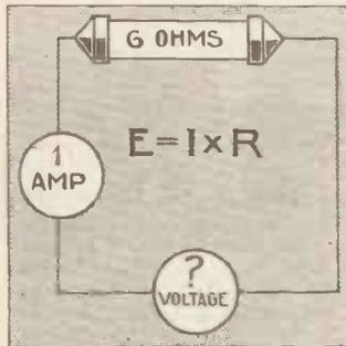
Knowing the current flowing through the circuit and the resistance of the circuit, you can readily find the voltage producing that current. Just another application of Ohm's Law
