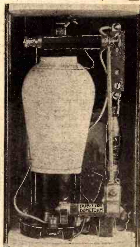
A close-up of the amplifier compartment of the "mike," in which the valve and its associate components can be seen
