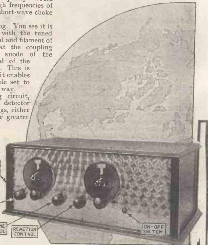
Control is very simple, all four wavebands being covered by the turn of a switch
