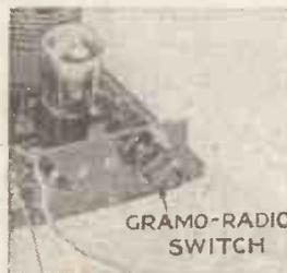
set the radio-gram switch wiring is in the detector circuit and the switch should be kept close to the detector holder, as shown here. The switch is seen mounted at the back of the set on a separate terminal strip near the detector holder
