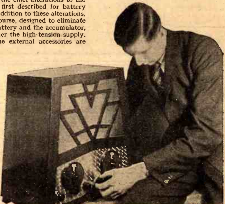
The "Melody Ranger" is a handsome instrument, designed to give the greatest efficiency. The lower part of the cabinet contains the actual receiver, and the loud speaker and mains unit are in a separate compartment above.
