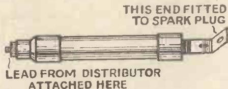
Fig. 1. The type of resistance for fitting to spark plugs
