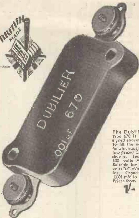
The Dubilier type 670 is designed expressly to fill the need for a high quality, low priced Condenser. Tested 500 volts A.C. Suitable for 250 volts D.C. Working Capacities .0001 mfd to .01 Prices from
