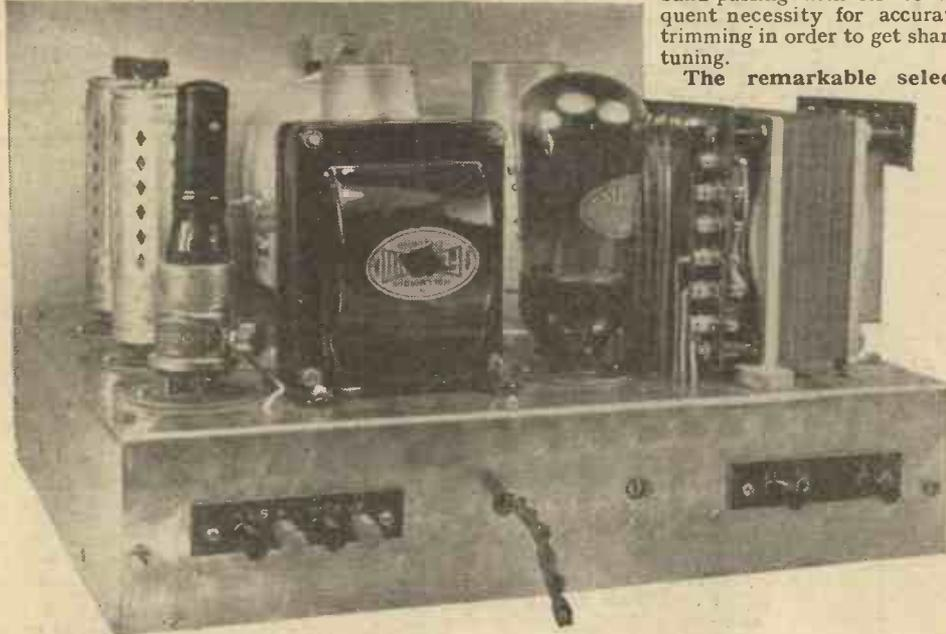
The basis of the receiver is a circuit consisting of variable-mu H.F. stage coupled by tuned-grid method to a screen grid detector which in turn is coupled to the power pentode output
