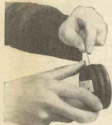
It is quite a simple matter to wind the quenching coils by hand as shown above
