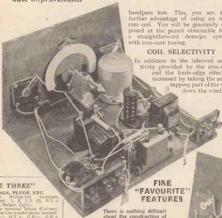
bandpass loss. This, you see, is a further advantage of using an iron-core coil. You will be genuinely surprised at the punch obtainable from a straightforward detector system with iron-core tuning.
