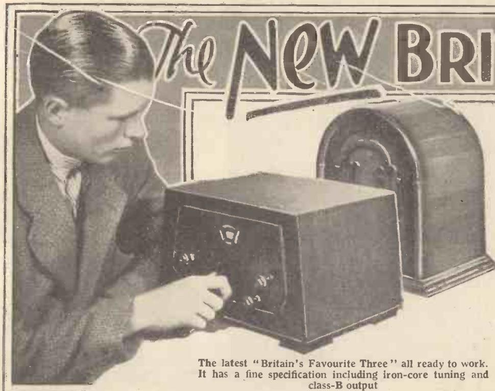
The latest "Britain's Favourite Three" all ready to work. It has a fine specification including iron-core tuning and class-B output
