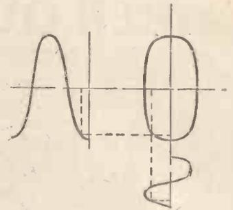
Fig. 7. An ellipse is produced when the voltages have different values at the same instant of time
