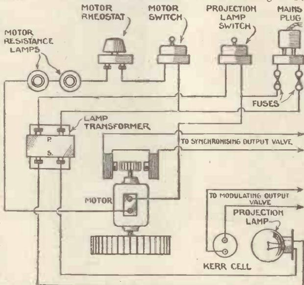
Fig. 3.—Here is the complete wiring for the television receiver
