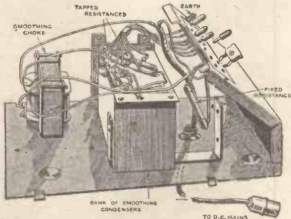
Typical of the Atlas range of mains units is this model DC15/25 for obtaining high tension from D.C. mains
