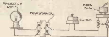
Fig. 2.—Connections for the projection lamp
