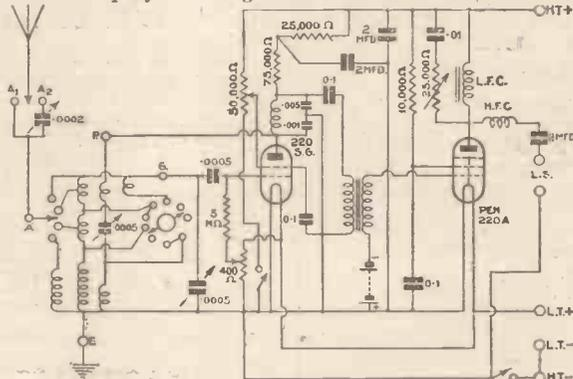
How to use the British General all-wave tuner in a "super-hot" two-valve circuit
