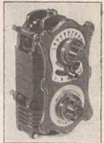
The British General tuning unit is built up on a most complex bakelite moulding
