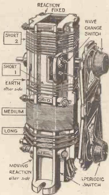
The British General tuning unit covers wave ranges of 14.5 to 40 metres; 32 to 90; 200 to 550; and 900 to 2,000 metres
