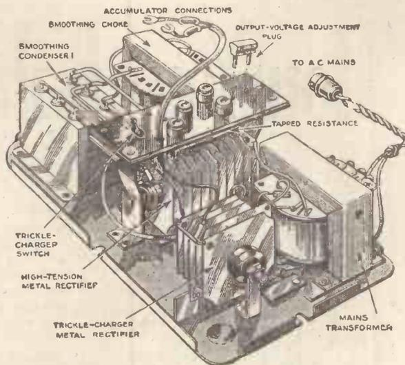
Ekco type K25 mains unit—another unit in the wide range made by E. K. Cole Ltd. for every purpose
