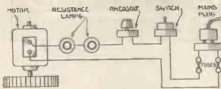
Fig. 1.—The connections for the motor
