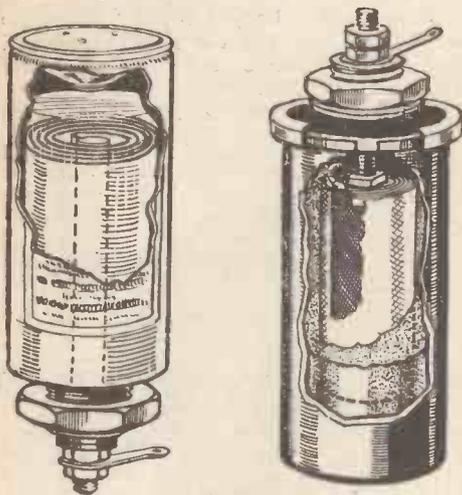
Typical electrolytic condenser constructions. (Left) Wet Dubilier, consisting of a coil of flat strip metal in electrolytic liquid, the centre pillar forming a contact, the case being earthed. (Right) Dry Telsens condenser with a roll of tinfoil and damp, impregnated linen embedded in beeswax, the foil being connected to the centre screw
