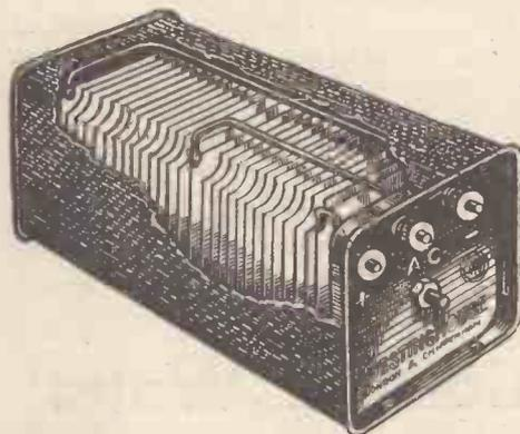
Typical Westinghouse high-tension rectifier with alternate copper and copper oxide plates
