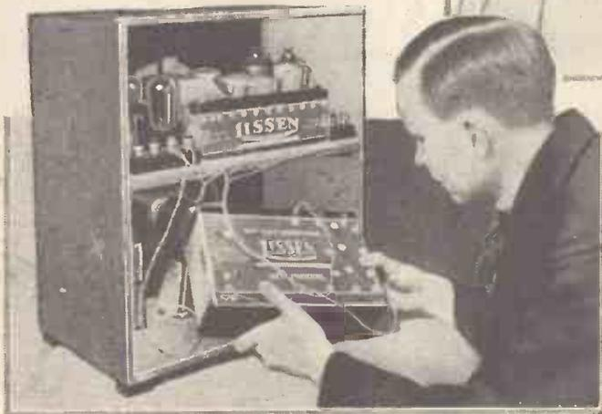
Putting the Ideal Four through its final tests before fixing the chassis in the console cabinet with loud-speaker
