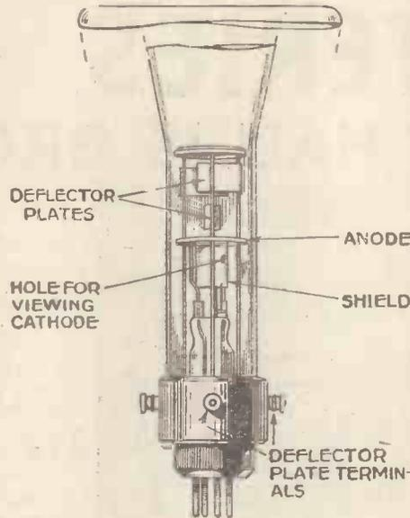
Fig. 3. The details of the electrode system of the cathode-ray tube
