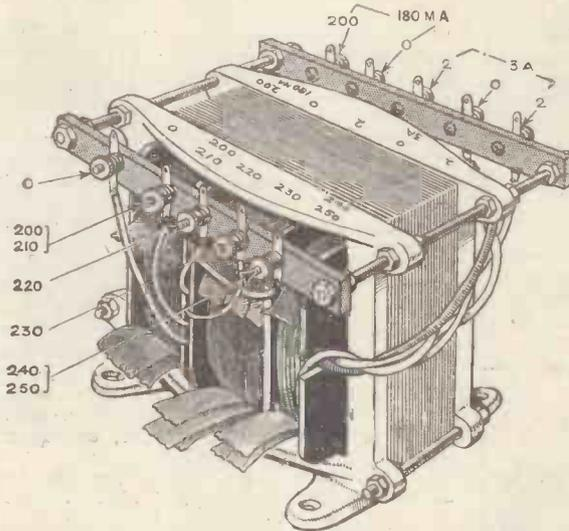
Constructional details of a typical mains transformer, clearly showing sectionalised windings, including filament output on the extreme right
