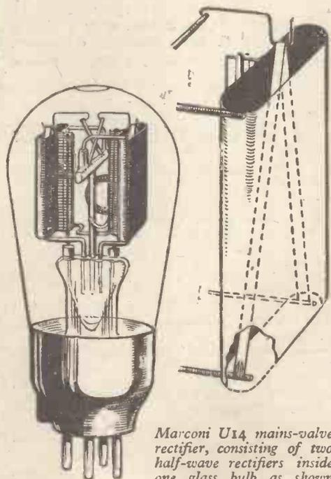
Marconi U14 mains-valve rectifier, consisting of two half-wave rectifiers inside one glass bulb as shown
