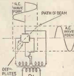
Fig. 6. The path of the beam when an A.C. voltage is applied to each pair of deflector plates with the voltages in phase
