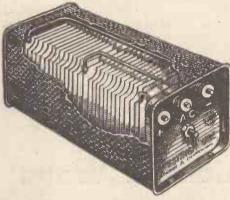
Typical Westinghouse high-tension rec: ifier with alternate copper and copper oxide plates
