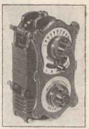
The British General tuning unit is built up on a most complex bakelite moulding
