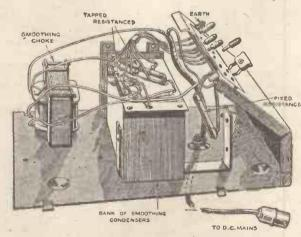
Typical of the Atlas range of mains units is this model DC15/25 for obtaining high tension from D.C. mains
