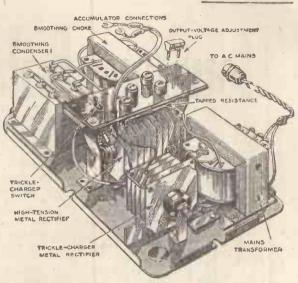
Ekco type K25 mains unit—another unit in the wide range made by E. K. Cole Ltd. for every purpose
