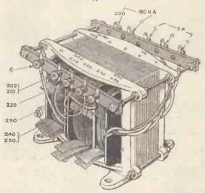
Constructional details of a typical mains transformer, clearly showing sectionalised windings, including filament output on the extreme right clearly
