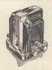
A sectional drawing of a typical iow-frequency transformer housed in a bakelite casing—a Lissen product
