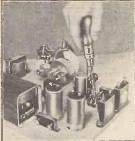
Using a ratchet screwdriver for fixing screws
