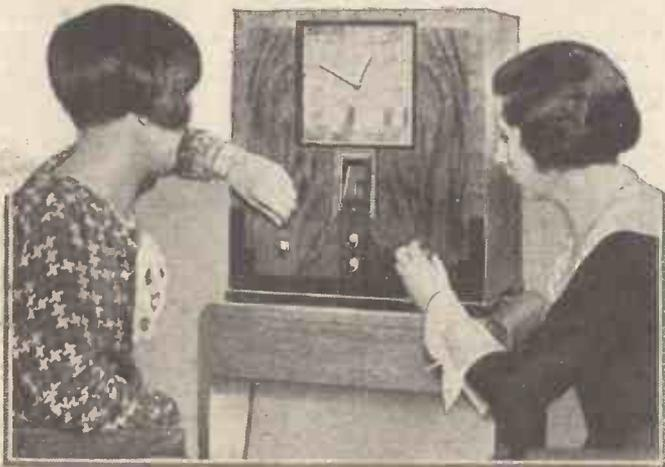
A central feature of the design of this H.M.V. Concert Seven super-het is an electric clock, which is ingeniously fitted into the loud-speaker fret
