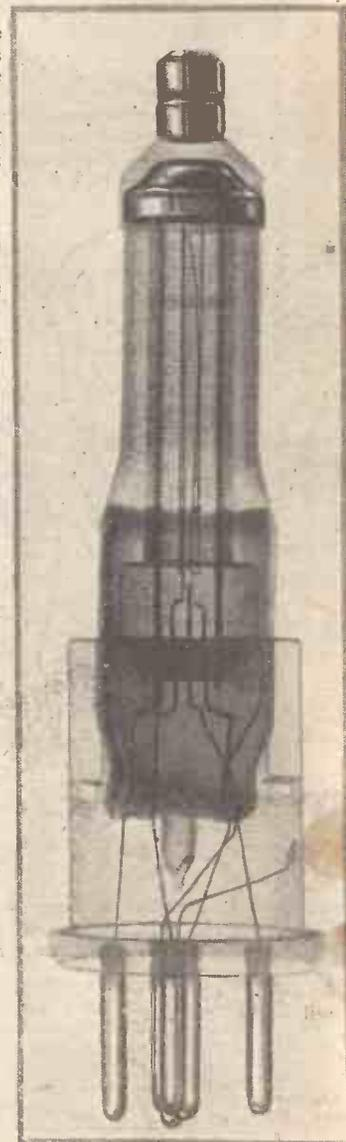
This X-ray photograph of a Catkin screen-grid type shows the construction of this unbreakable valve
