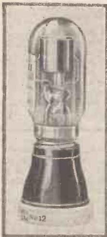
One of the neon discharge tubes used in the timing circuit of a road traffic light of the Electromatic type
